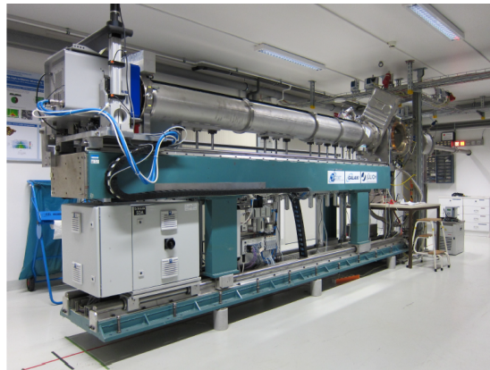
Figure 5.7: GALAXI diffractometer for GISAXS and XRR measurements. Taken from [71].
