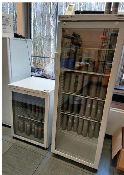
**Figure C.1.** Incubator with soil samples (280 PVC tubes).
