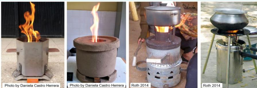
**Figure 1.15.** Examples of top-lit up-draft microgasifiers.
