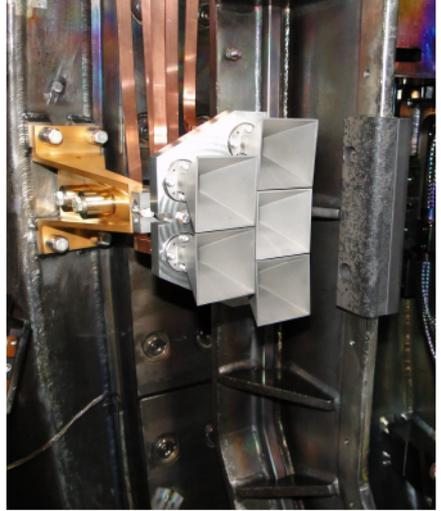
Figure 5: Photograph of the installed correlation reflectometry antenna at AUG. The middle antenna in the right column launches the microwave and the surrounding antenna measure the reflected signal.
