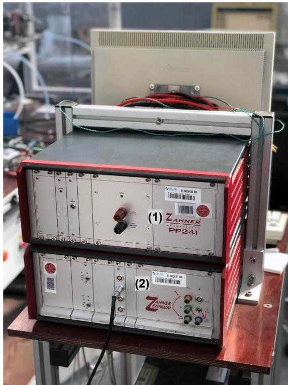
Figure 3.10: EIS electrochemical workstation, (1) Zahner PP241 power potentiostat, (2) Zahner Zennium device.
