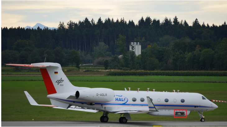
Figure 3.2: The German High Altitude and Long Range Research Aircraft (HALO) during the WISE campaign with GLORIA (red rectangle), mounted in the belly-pod and looking from the right side of the aircraft. Photo by Peter Preusse.
