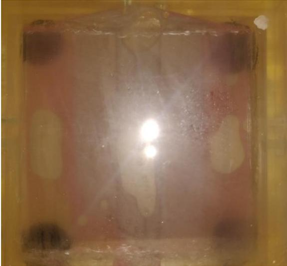
**Fig. 4.51** Fracture after injection of silver coloured water
