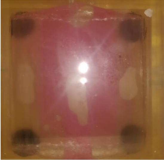
**Fig. 4.49** Fracture after injection of magenta coloured water
