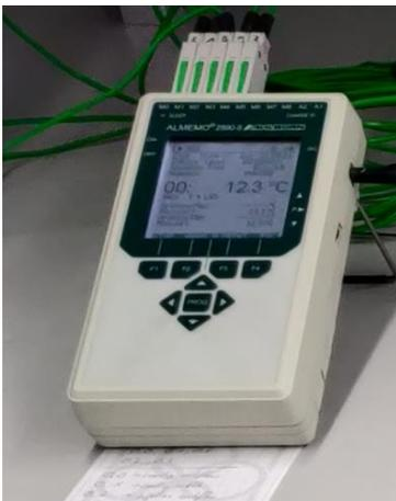
**Fig. 4.41** Data acquisition system
