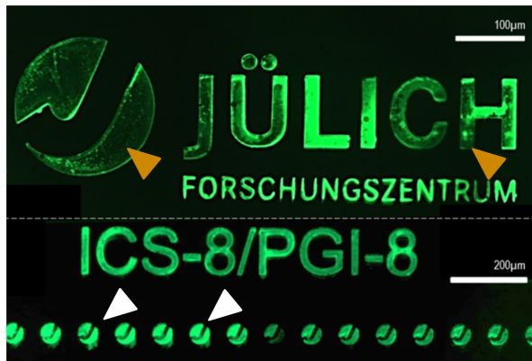
Figure 4.18: Inhomogeneities in the transferred protein patterns. Protein pattern is visualised via the FITC fluorophore that is covalently linked to the PLL. Orange arrows indicate a bad protein transfer that resulted in a blank area without protein. White arrows indicate smeared protein.
