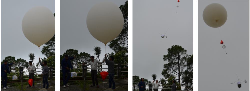
Figure 2.1: A balloon launch on a cloudy day at Nainital base camp. Test flights were launched in July 2016 under the supervision of Peter Ölsner from GCOS Reference Upper Air Network (GRUAN) [Dirksen et al., 2014].
