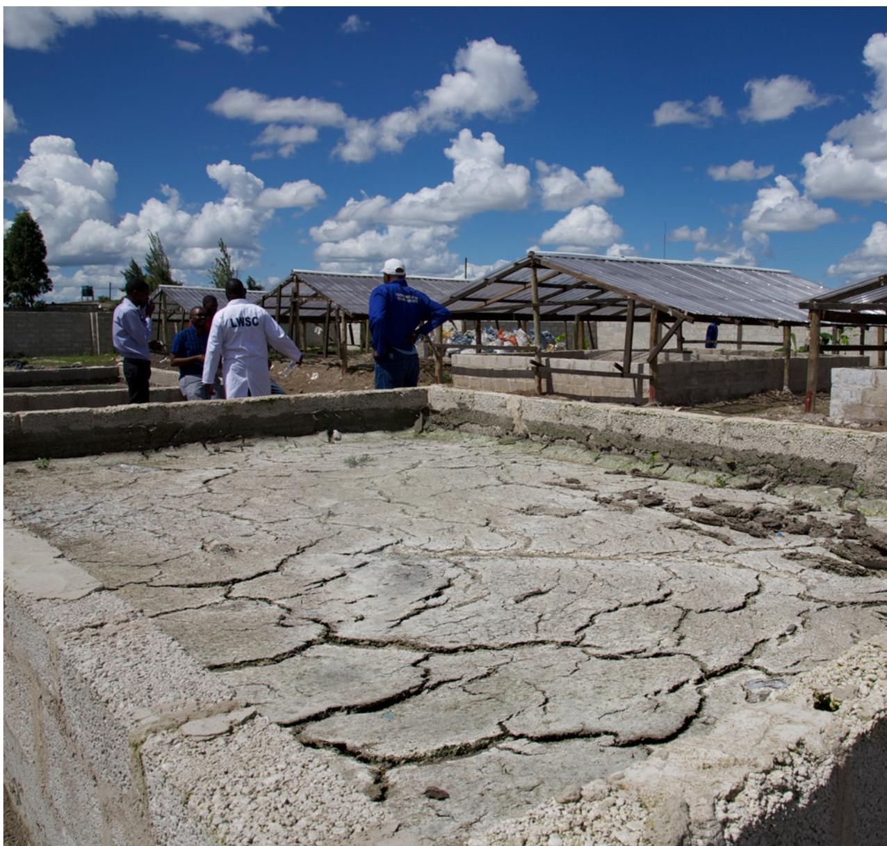
Above: Trials for the design of faecal sludge treatment facilities in Lusaka
