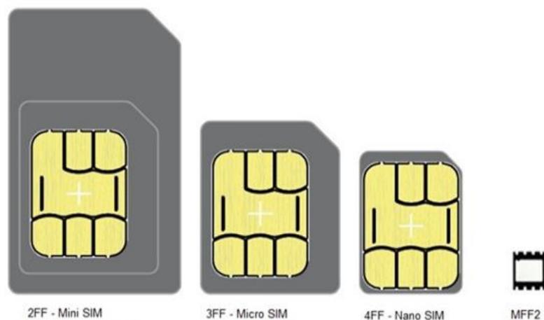
Source: ISO/IEC 7810:2003, ID-000 for 2FF; ETSI TS 102 221 for 3FF and 4FF; ETSI TS 102 671 for MFF2. Graphic by EMnify.
