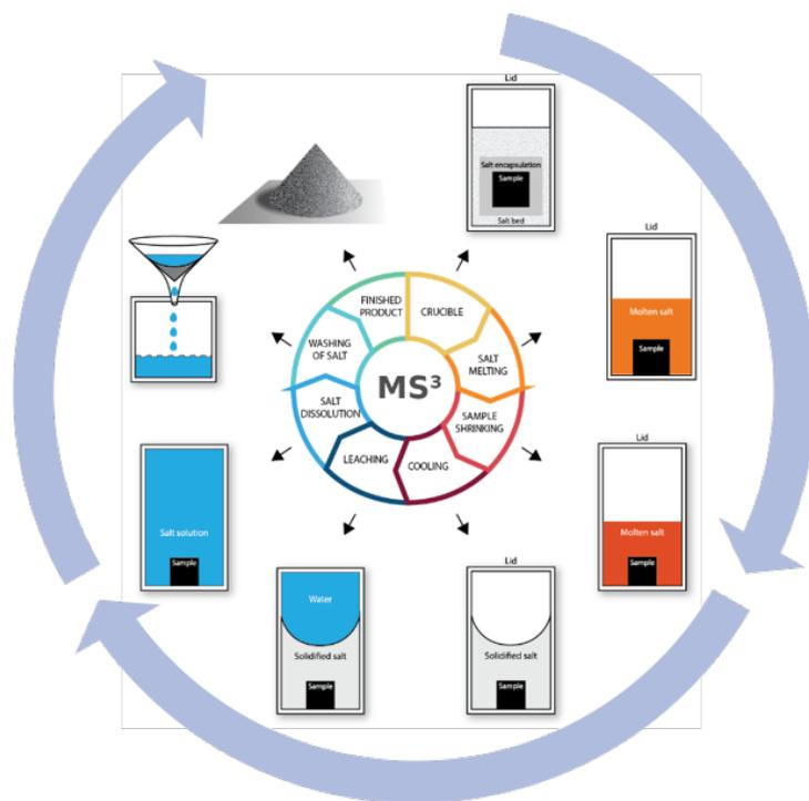
Figure 4.1: Schematic of molten salt shielded synthesis ( $MS^3$ ).
