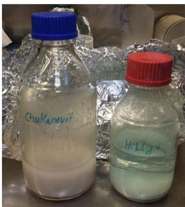
**Fig. 4.4** Chukanovite (left) and Fe-Hibbingite (right)
