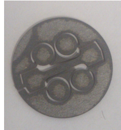
Figure 6.4: Two sample geometries were installed and irradiated with 3 MeV protons. The first is an established plasma exposure sample geometry while the geometry on the right is for comparison with high energy proton irradiations.
