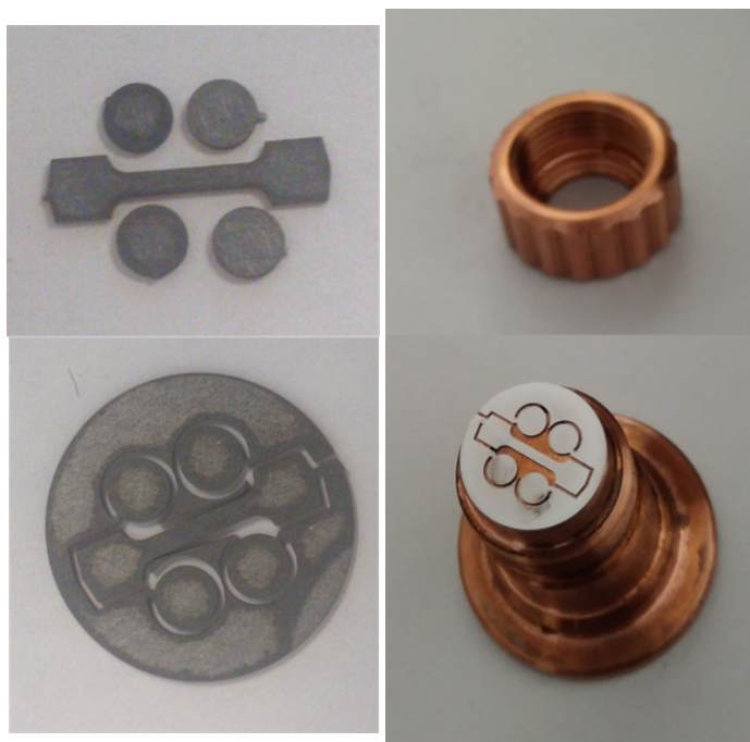
Figure 7.9: 1 st trial of the sample holder with the plain sample on the Cu sample holder.
