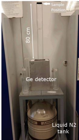
Figure 8.8: The gamma detector system and its calibrated efficiency curve using isotopes of known activity and specific high intensity gamma lines. The detector was calibrated for 80 cm.
