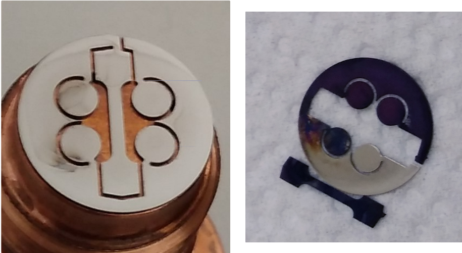
Figure 8.7: Sample before irradiation (left) polished to 1 \mu\text{m} and post irradiation (right) with an oxide layer.
