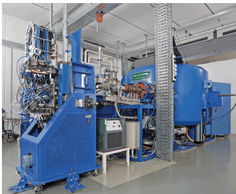
Figure 7.1: BC1710 aka Baby cyclotron located at the institute for nuclear chemistry and routinely used for the production of radio-isotopes such as ^{18}\text{F} and ^{11}\text{C} .
