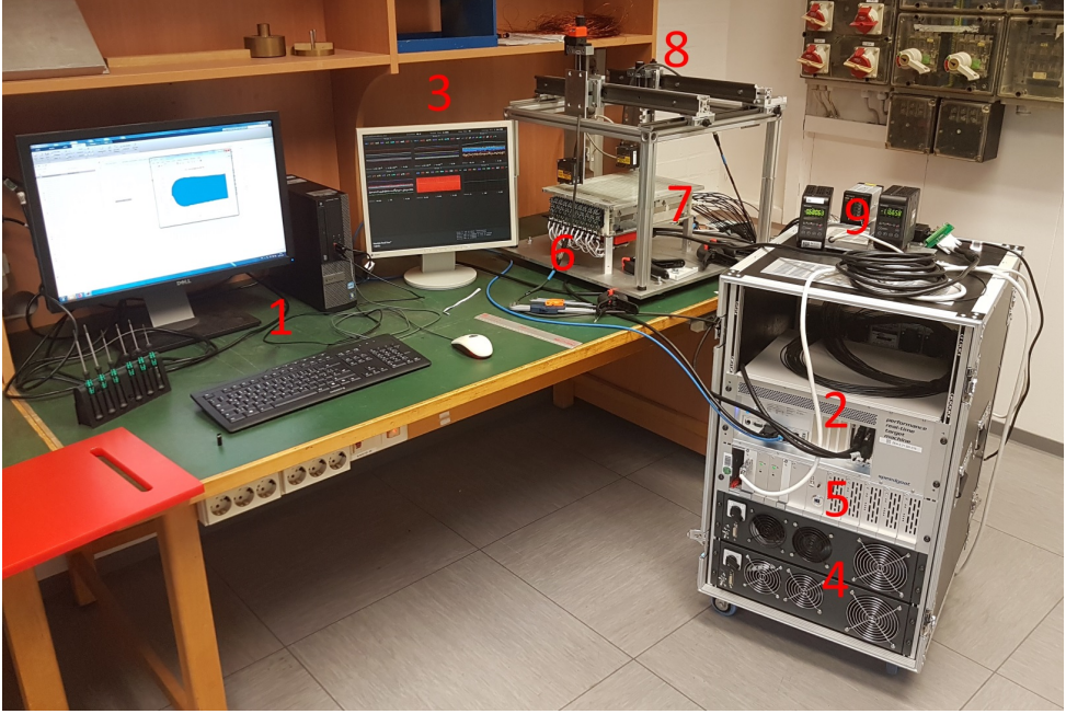
Figure 3.1: The test stand with tools and the actuator system 2.1 (see also Chapter 4). The development computer (1) is a desktop PC running a windows OS and Matlab Simulink. It is connected via Ethernet LAN (Local Area Network) to the Speedgoat Performance Target computer (2), which shows important data on the connected screen (3). In the same box, there are also racks containing amplifiers (4, see Section 4.3) and power supplies (5) for sensors (6, see Section 4.2). Finally, there are the actuator system (7) and a frame holding the position reference sensors (8), whose readout electronics are placed on top of the box (9).
