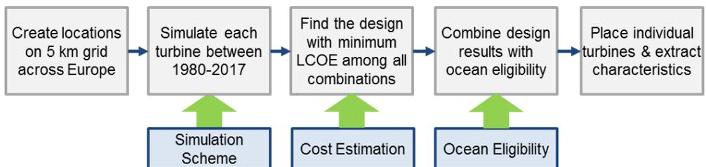
Figure 3-6 Overall workflow used in the optimal turbine design analysis.
