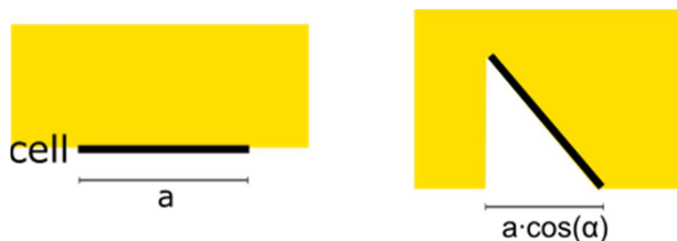
Figure 7.9: Illumination conditions at the current-voltage measurement setup for the evaluation of the influence of varied incident angles. The effective illuminated device area changes according to cosine law (44), taken from reference [132] .
