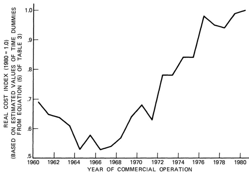
*Notes:* This figure reproduces Figure 2 from Joskow and Rose (1985). It plots the index of real costs per kilowatt of installed capacity associated with the construction of coal-burning electricity generating units. Notice that it declines during the early 1960s, stabilizes in the mid 1960s, and then increases starting around 1966 to a level that by 1980 is substantially higher than the level in 1960.
