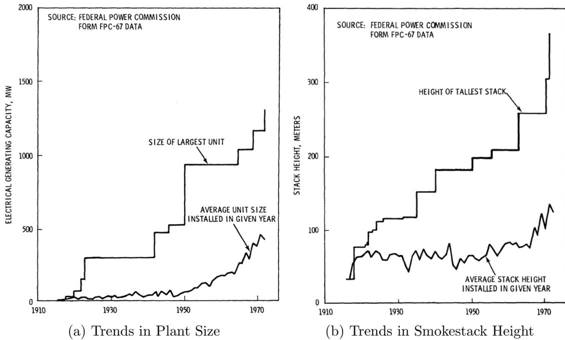
*Notes:* This figure displays trends in plant size and smokestack height. Panel (a) documents the average and maximum capacities (in MW) of electricity generating units in each year. Panel (b) documents the average and maximum smokestack height (in meters) of electricity generating units in each year. The data used to construct these figures come from Federal Power Commission Form FPC-67. *Source:* Figures 3 and 4, EPA (1976c).
