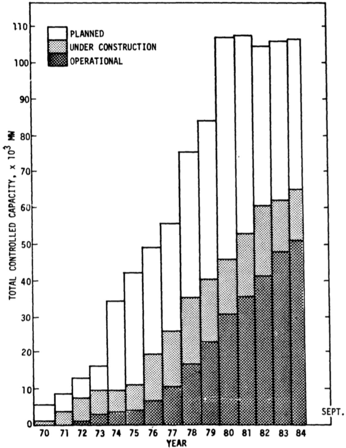
Notes: This figure presents a historical breakdown of utility status reports for operational, under construction, and planned flue gas desulfurization (FGD) capacity – December 1970 through September 1984. Source: Figure 2, EPA (1984).
