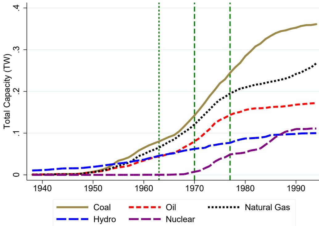
*Notes:* This figure documents annual national total electricity production capacity by fuel type. The data underlying this figure come from the EIA Form 767. The thin dashed vertical green line represents the Clean Air Act of 1963 while the thicker green vertical lines represent the 1970 Clean Air Act and its amendments in 1977.
