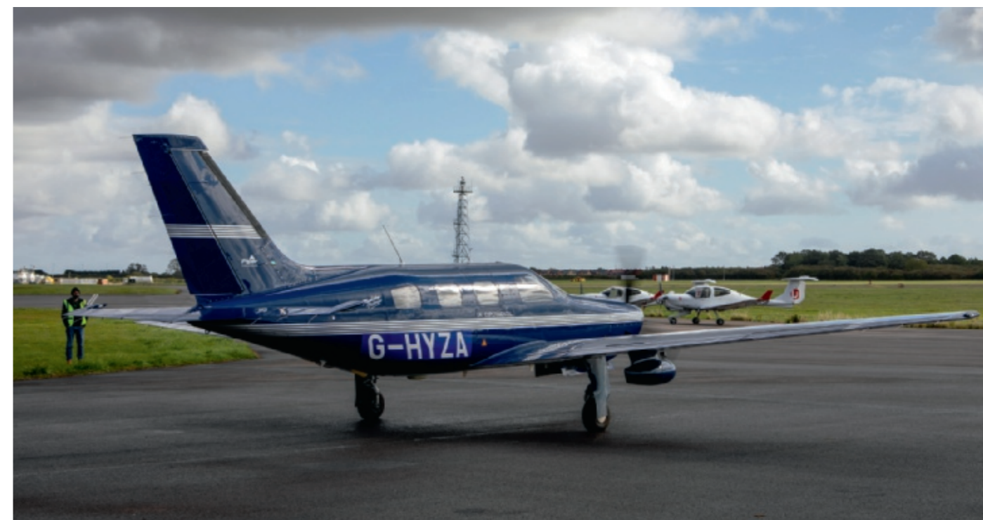
SMALL WONDER: ZeroAvia's six-seater aircraft is powered by a hydrogen fuel cell.
