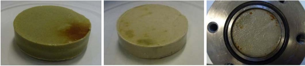
**Fig. 2.11** Rust traces on the bottom side of unreacted B09 (left) and B23 (middle) pellets and on the porous steel plate in contact with B11 (right, no rust on B11 observed) after permeability measurements
