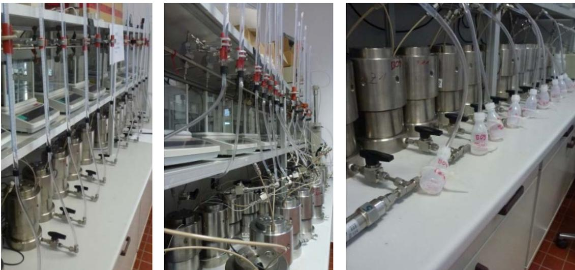
**Fig. 2.5** Burettes used to supply VGH to permeameter cells from cell bottoms (left) and cell tops (middle) and by a valve pump to measure the permeability (right, regard plastic vessels connected to cell tops to collect solutions percolating through bentonite pellets)
