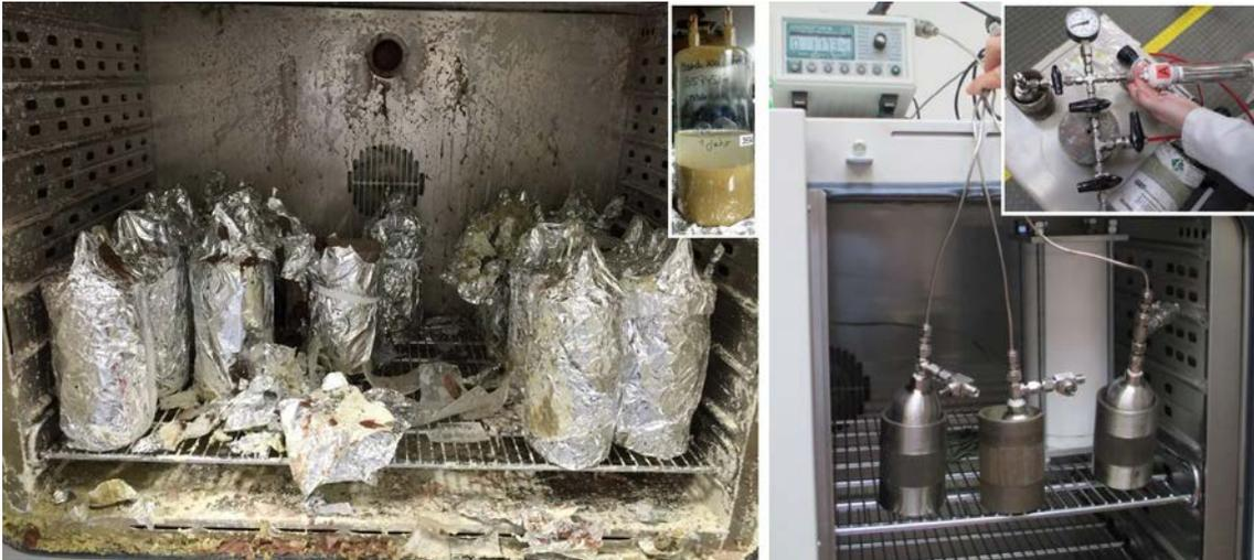
**Fig. 2.2** Left: disrupted and intact welded glass vessels in a drying oven after several hours of heating at 120 °C (inset: a welded glass vessel without aluminium foil). Right: alloy vessels with tubing to pressure transducers outside the oven and a gas sampling valve at the head piece (inset: gas sampling)
