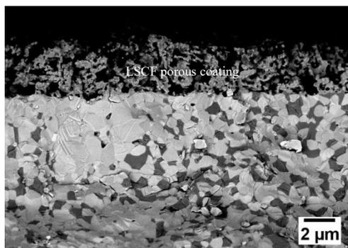
Figure 7.9 Cross section of the coated CF-D.
