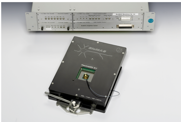
Figure 3.4: Picture of the BioMAS measurement setup consisting of the main-amplifier (top) and the pre-amplification headstage (bottom, black) including a MEA with electrolyte and reference electrode (green center).
