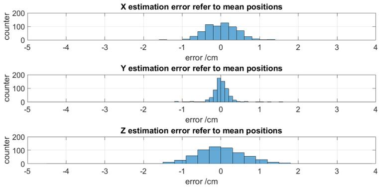
**Figure 4.20:** Estimation error statistics in 3 directions (X,Y,Z).
