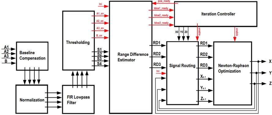
Figure 4.6: Block diagram of the processing core sub-system.
