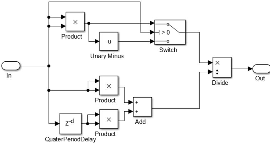
Figure 3.30: Simulink model for the proposed normalization sub-system.
