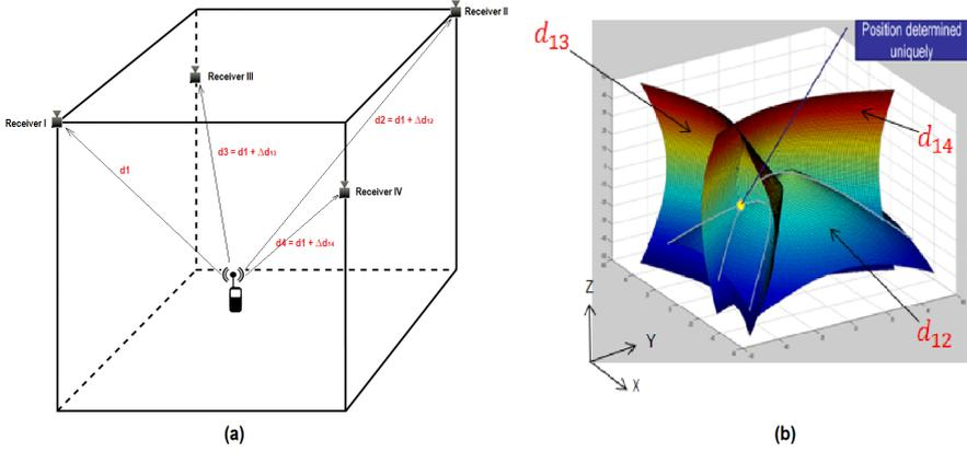
**Figure 3.16:** Example sensor network for a hyperbolic position fix indoor positioning system. RF receivers are placed at known positions (left). The target emitter is located by TDoA information of pairwise receivers (right).
