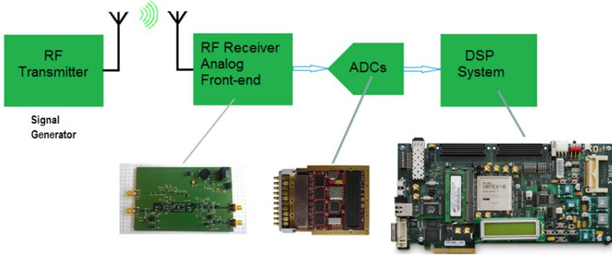
**Figure 3.9:** Block diagram of the signal chain components.
