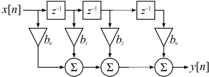
**Figure D.1:** FIR filter direct form diagram
