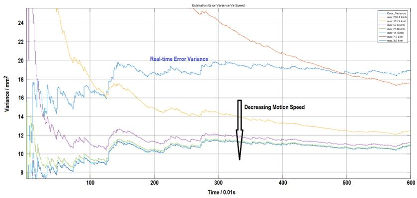
Figure 3.39: The filtering performance is improved with a slower motion.
