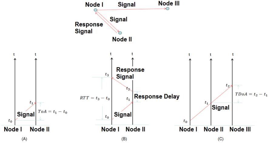
**Figure 2.6:** Time measurements: time of arrival (ToA) (A), round trip time (RTT) (B), time difference of arrival (TDoA) (C).
