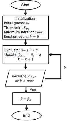
**Figure 3.37:** Flow chart of the proposed iterative estimation process.
