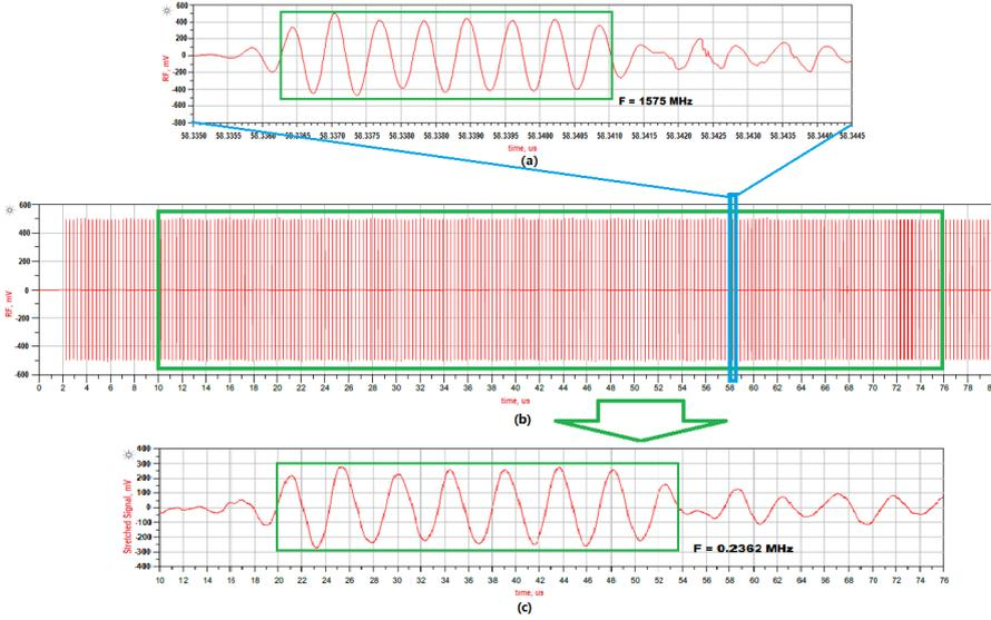
**Figure 3.24:** Example simulation result of the signal stretching. (a) refers to one segment of the received periodic RF signal (b). (c) is the stretched signal by sub-sampling the received signal (b).
