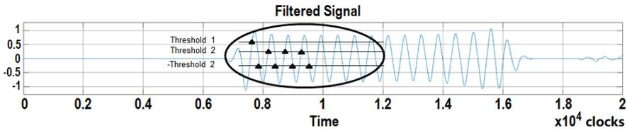
**Figure 3.34:** The normalized signal is filtered by the designed FIR low pass filter. Original signal (up), normalized squared signal (middle) and filtered signal (down), two thresholds are introduced to determine a event.
