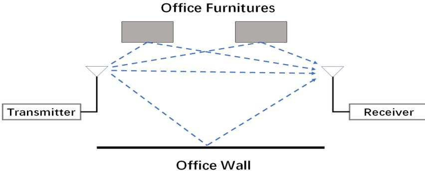
**Figure 3.3:** Multipath propagation in an indoor environment.
