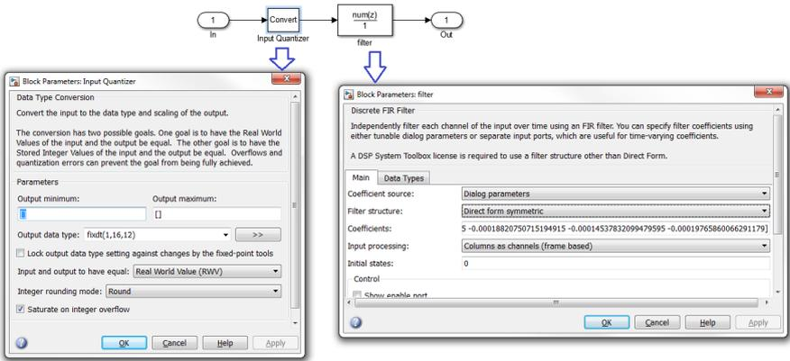
**Figure D.3:** Realize the designed filter in Simulink, including two basic modules: a filter and a quantizer.
