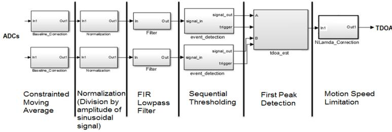
Figure 3.27: Simplified signal processing chain
