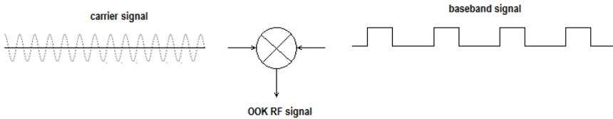
**Figure 3.10:** The transmitter emits periodic OOK modulated signal.
