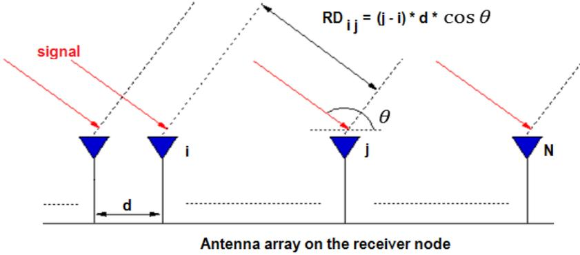
**Figure 2.5:** Angle estimation using antenna array.
