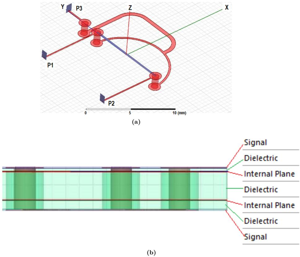
**Figure 3.22:** (a) Employed power combiner with signals input from p1 and p2 then output from p3. (b) PCB layers stack structure with conductor of copper and dielectric material of FR-4.
