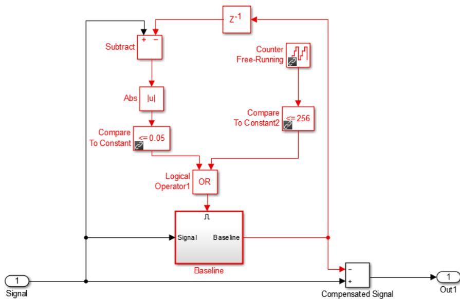
Figure 3.28: Baseline Estimation Subsystem, average 64 restricted samples
