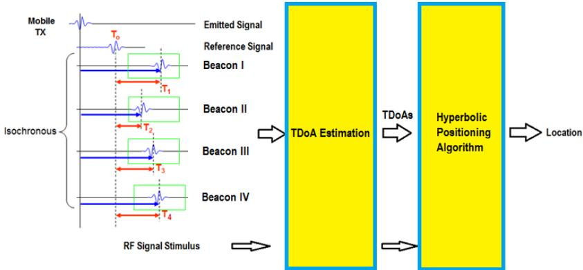
Figure 1.1: Simplified signal processing chain
