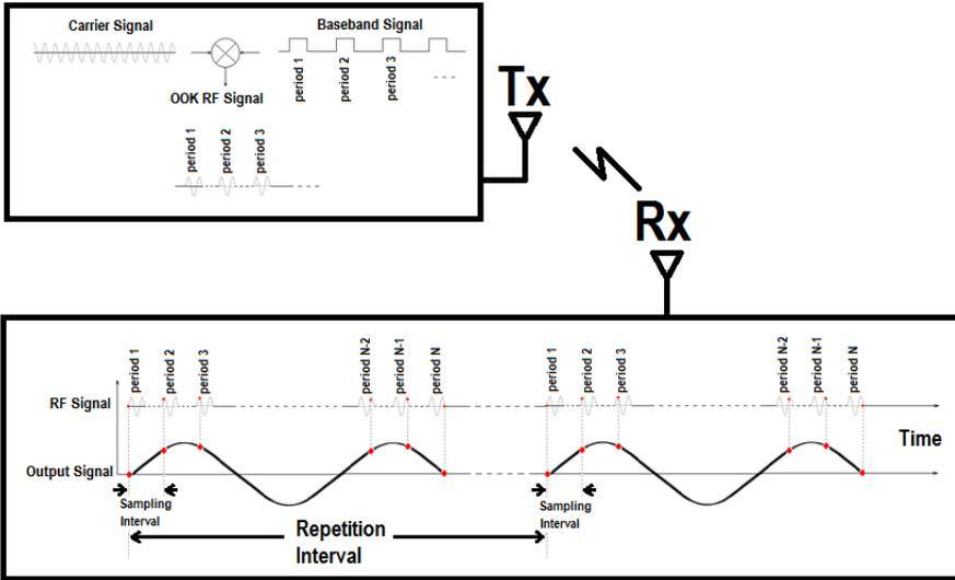
**Figure 3.17:** Reconstruction of one wavelet from  $N$  signal periods. The transmitter emits OOK modulated signal. The receiver reconstructs one period signal from sampling  $N$  periods (in analog domain).
