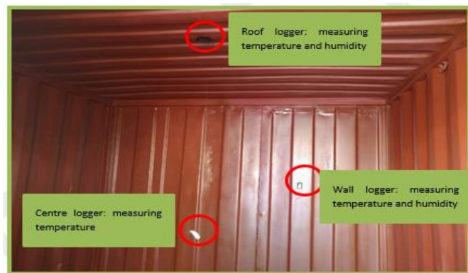
Figure 9: Configuration of logger placement in the container
