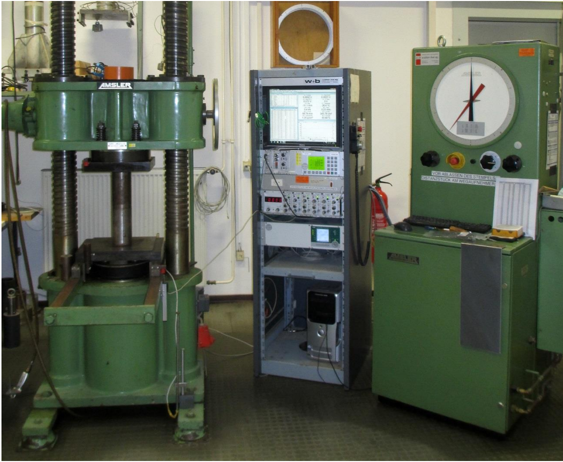
Fig. 6.2 Amstler hydraulic press for compaction of the samples
