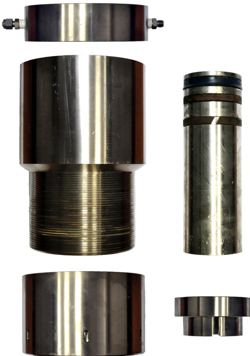
Fig. 5.2 Photos of the different parts of the diffusion cell Left row from top to bottom: top flange, body, sleeve nut Right row from top to bottom: plunger, centering ring
