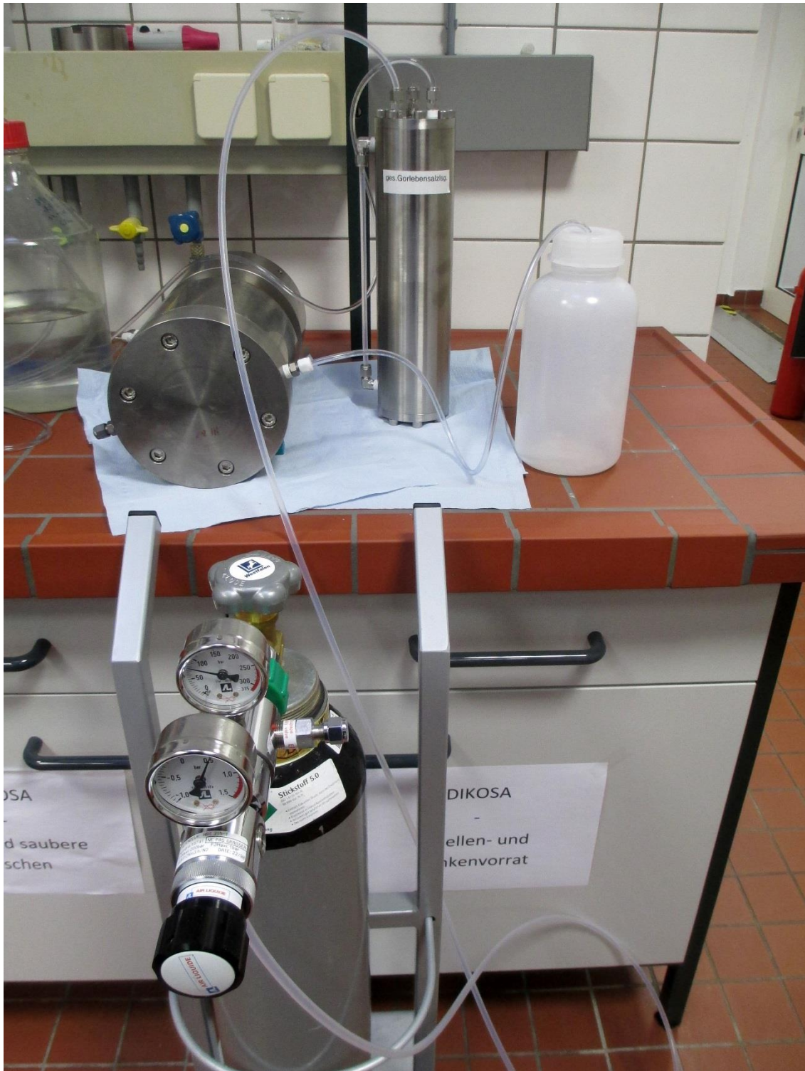
Fig. 6.5 Experimental setup during sample saturation and permeability measurement
