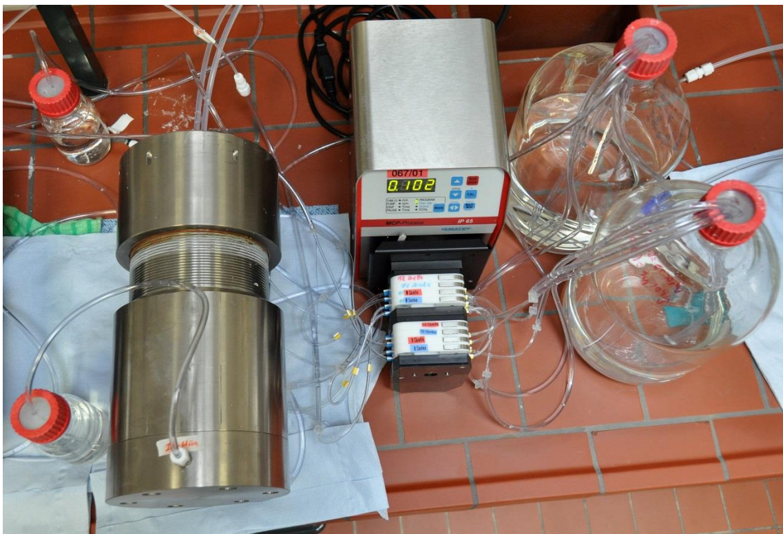
Fig. 6.7 Photos of the diffusion experiment setup from front and above The large bottles are the inlet reservoirs, while the small bottles are the outlet reservoirs
