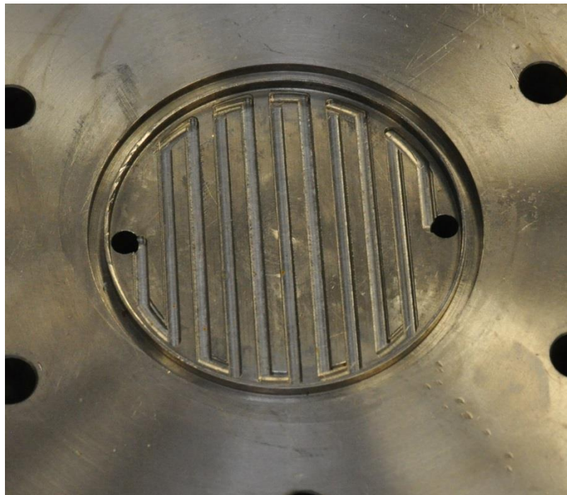
Fig. 5.4 Detail view of milled surface in the top flange
