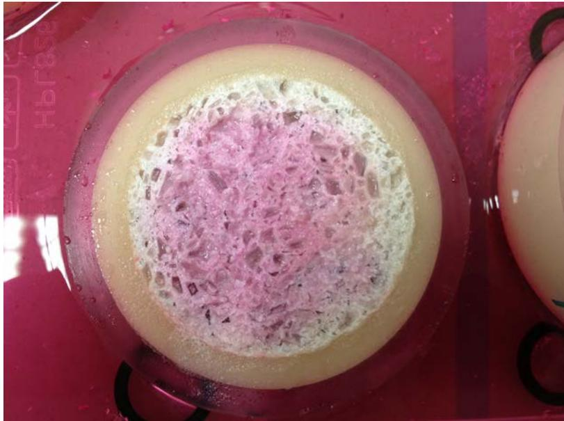
**Fig. 4.37** Sorel concrete sample from through-diffusion experiments in coloured tracer solution. The violet colour occurs in the middle of sample only verifying that diffusion occurred in the concrete matrix
