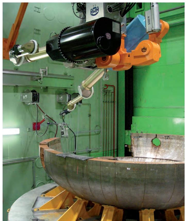
*Fig. 29b: Chamber for dry cutting*
