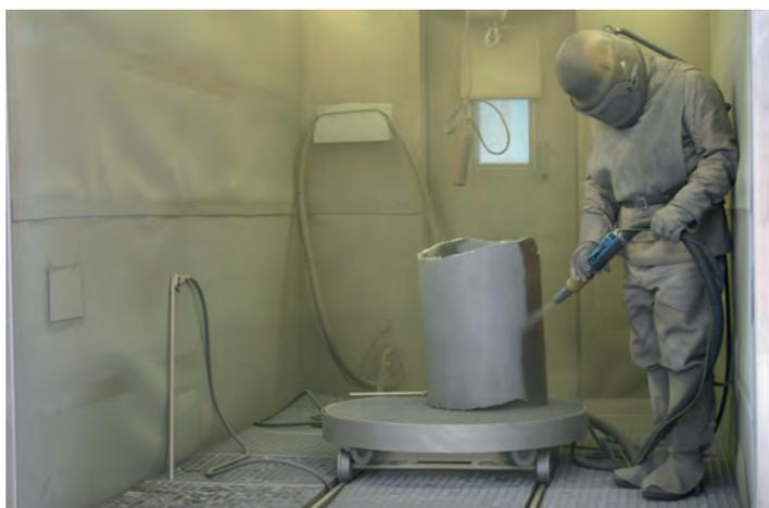
**Fig. 16:** Decontamination by sandblasting
