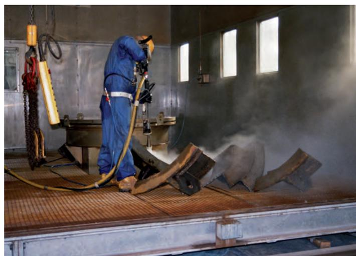
**Fig. 26:** Decontamination by high-pressure water jet cleaning
