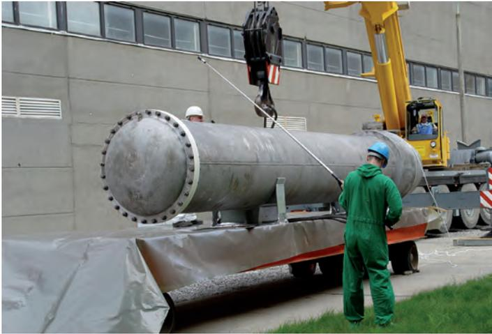
*Fig. 39: Dose rate measurement*
