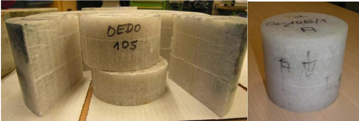
**Fig. 2.45** Crushed salt core D-OE-105/01 with sample remains, and the core after the triaxial compaction/permeability test
