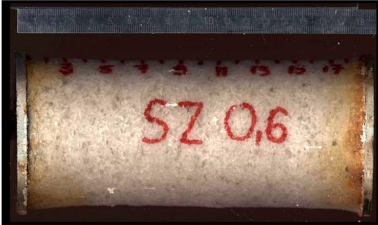
**Fig. 2.24** Sample with 0.6 % initial moisture content after dismantling
