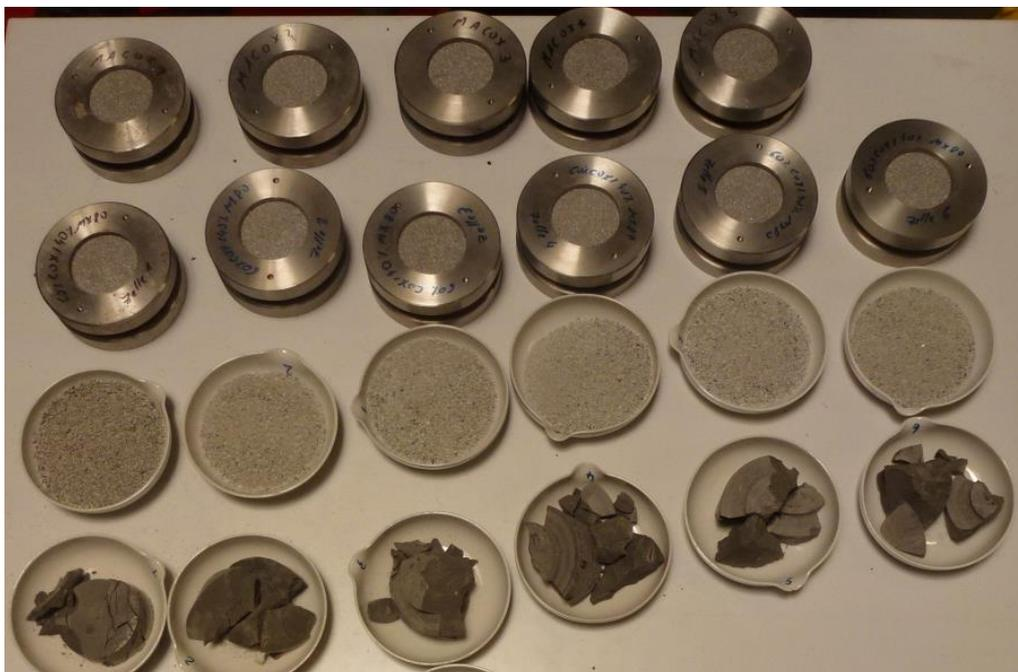
b) Samples in test group III: confined in cells and unconfined
