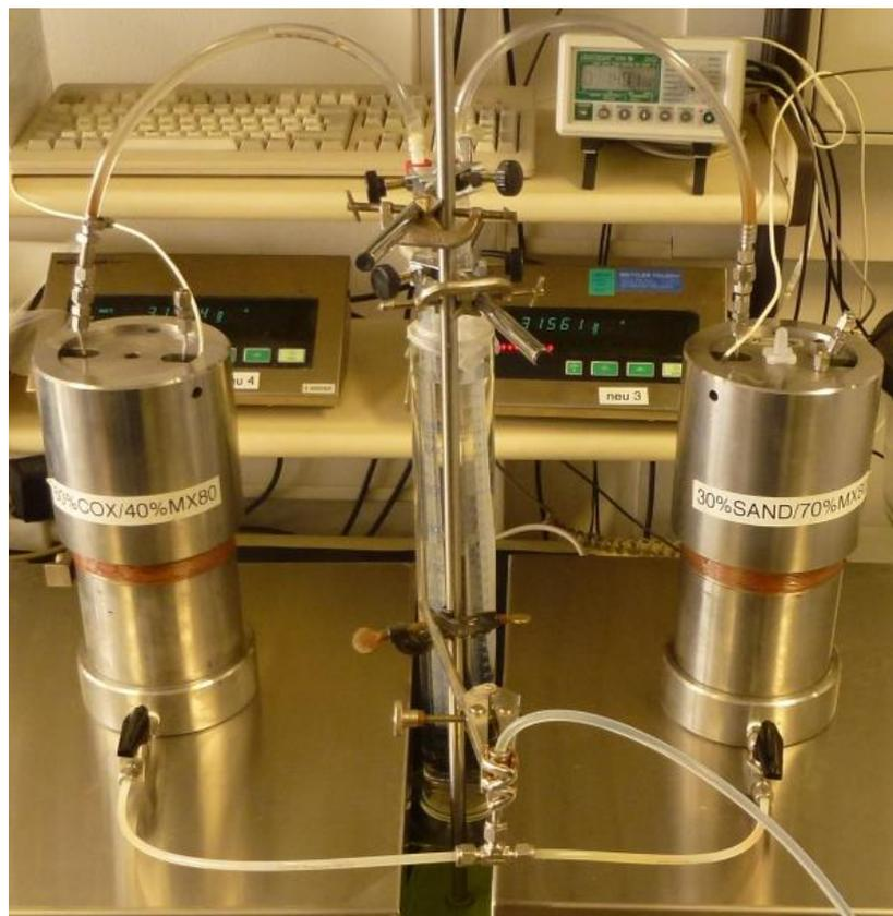
b) Setup of borehole sealing tests
