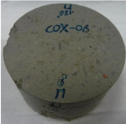
a) Compacted crushed claystone
