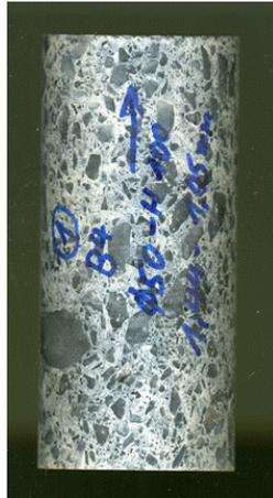
**Fig. 4.1** Salt concrete sample
