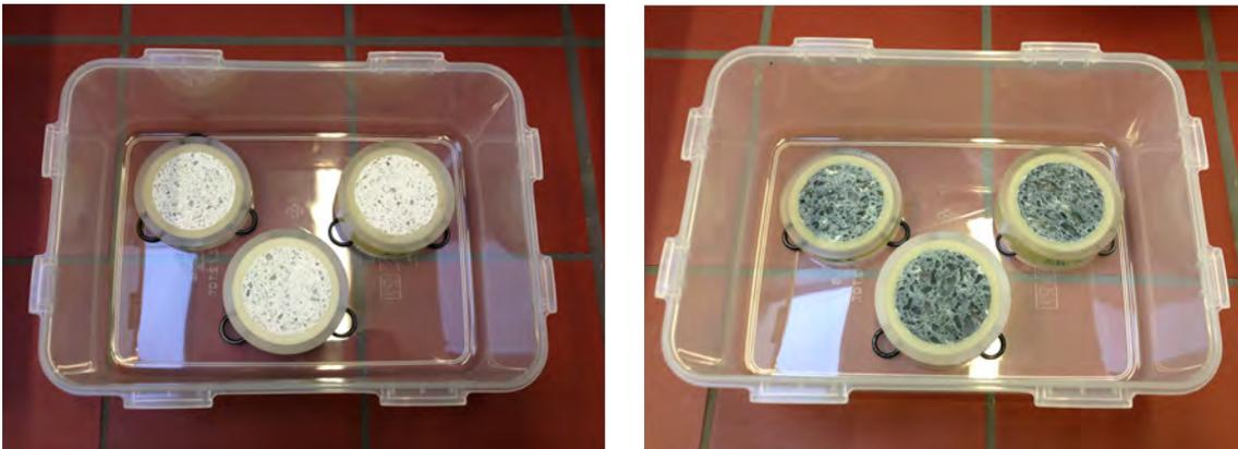
**Fig. 6.16** Samples in first phase of through-diffusion experiments before solutions were admitted. Sorel concrete (left) and Salt concrete (right)
