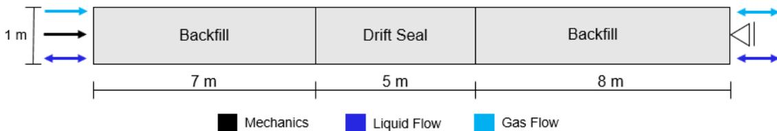
**Fig. 6.1** Model geometry and considered processes for the third modelling phase
