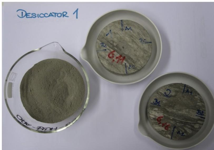
**Fig. 4.1** Pictures of the powder and disc samples from borehole BDM-B9 for measurement of water retention properties
