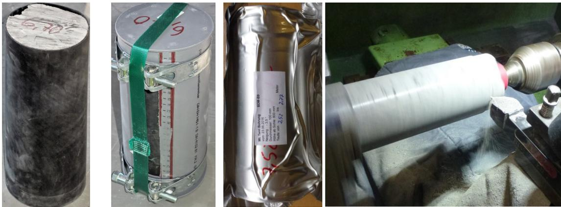
inserted in jacket    confined in cell    confined in cell    prepared to cylindrical sample in a lathe
