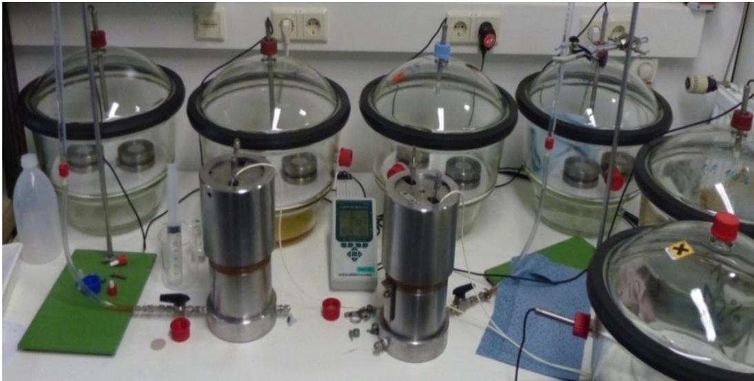
**Fig. 4.3** Measurement of water retention properties of the samples in desiccators at different relative humidities
