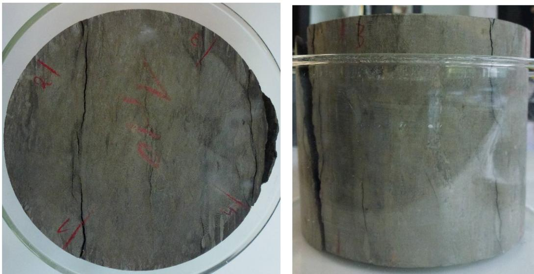
**Fig. 2.8** Wetting-induced cracks along bedding planes in an unconfined sample (diameter = length = 100 mm) at relative humidity of 100 % over 6 months
