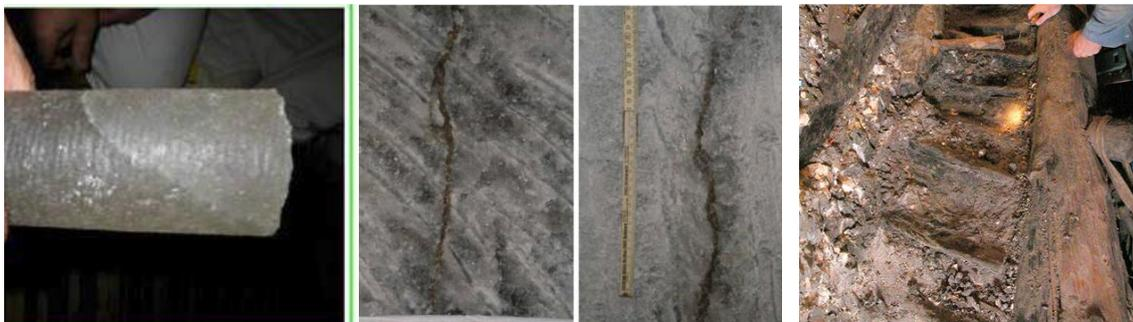
**Fig. 4.21** Technical analogues from mining and geological analogues for convergence and self-sealing of rock salt
