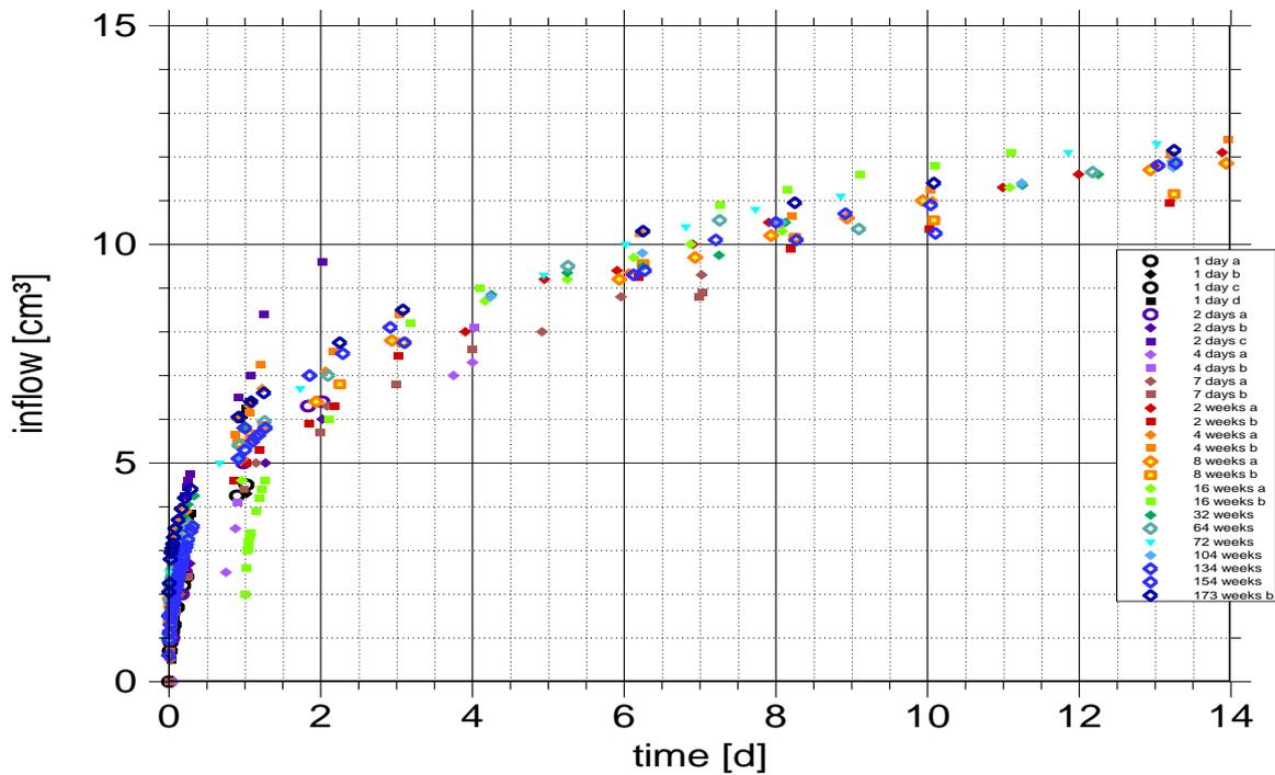
Fig. 4.12 Accumulated water mass for 26 tests during the first 14 days (old set-up)
