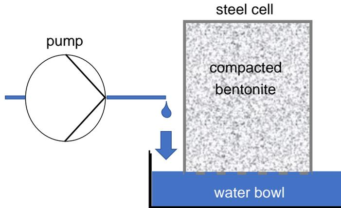
**Fig. 4.2** Test principle for direct inflow control via water bowl
