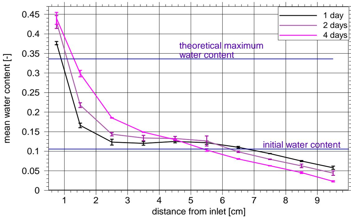
**Fig. 4.9** Mean water content distributions for running times of 1, 2 and 4 days
