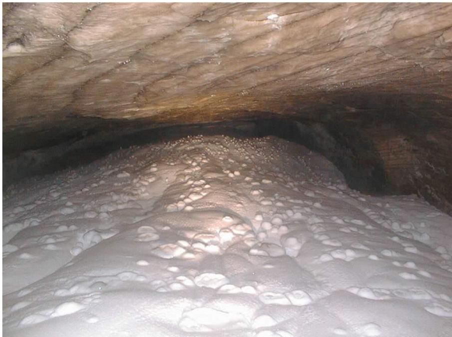
**Fig. 4.20** CO<sub>2</sub> glacier after an underground gas breakout in salt rocks /MIN 14/
