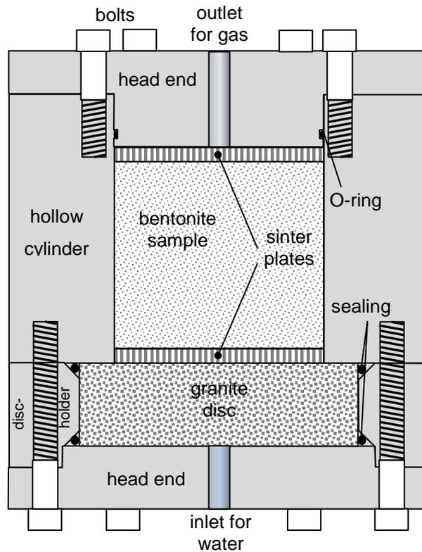
**Fig. 4.1** Test cell for inflow reduction by low permeable porous material
