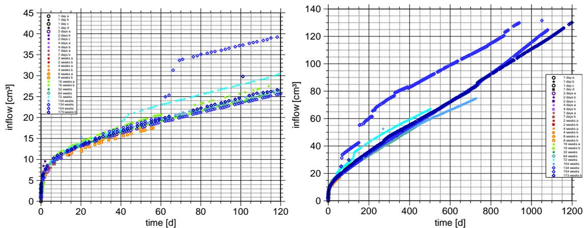
Fig. 4.13 Accumulated water mass for 26 tests during the first 120 days (left) and 600 days (right) (old set-up)
