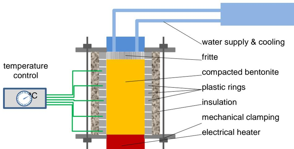
**Fig. 4.6** Principle of the test set-up
