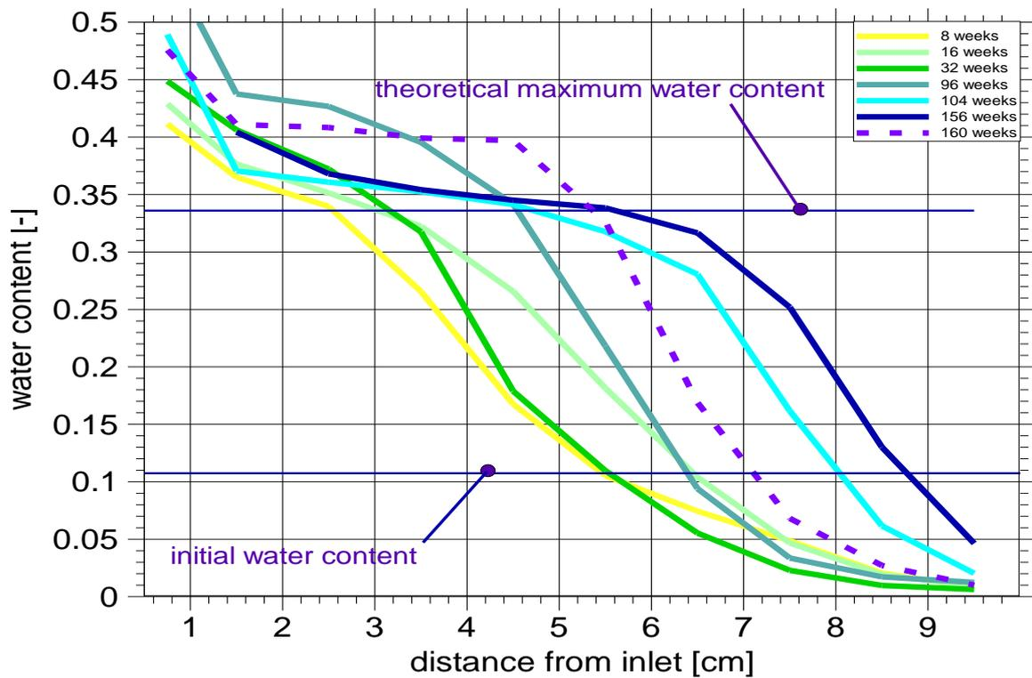
**Fig. 4.14** Water content distributions determined with the new test set-up
