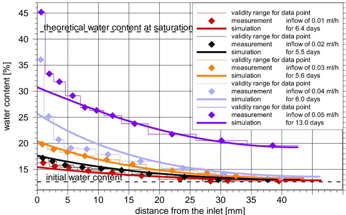
**Fig. 4.4** Measured and calculated water content distributions varying the inflow rate
