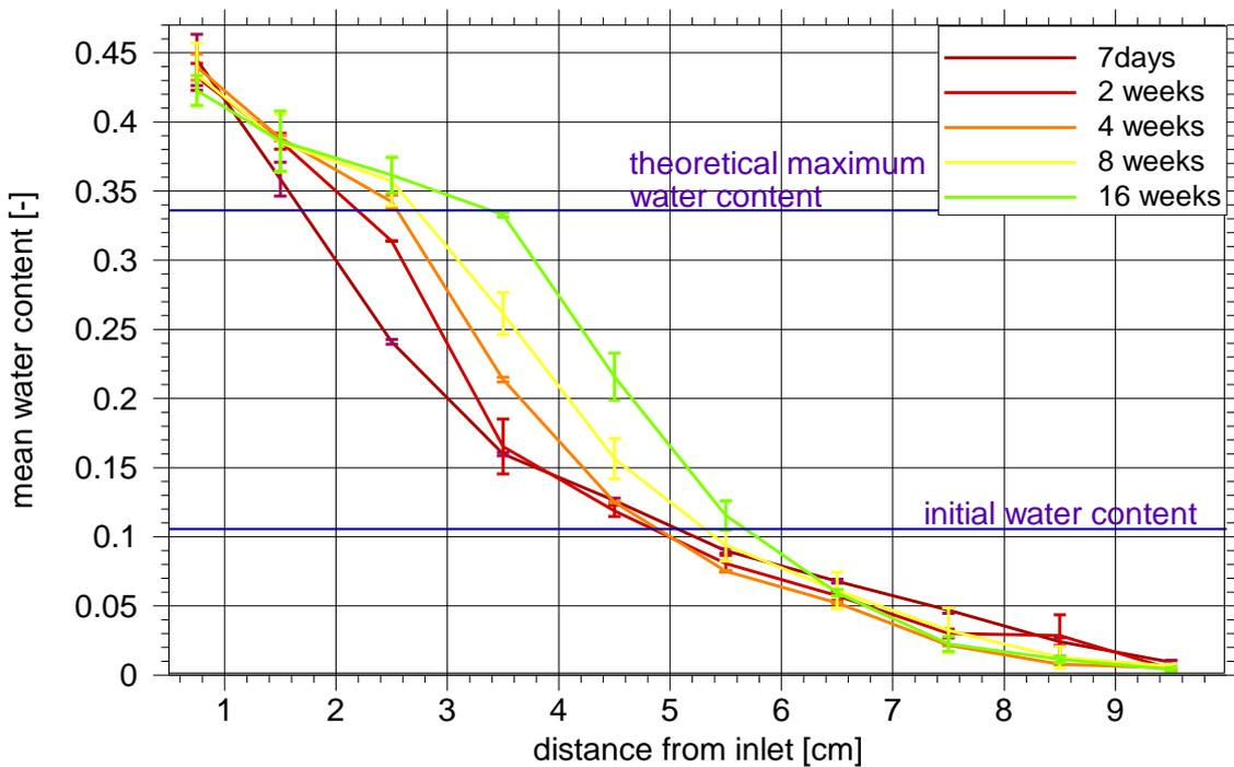
**Fig. 4.10** Mean water content distributions for running times of 1 to 16 weeks
