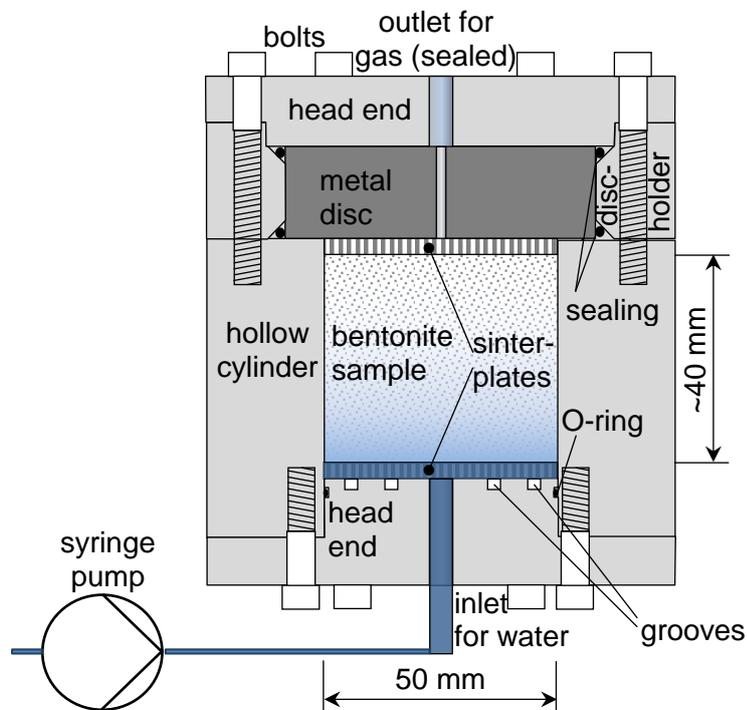
**Fig. 4.3** Final test setup
