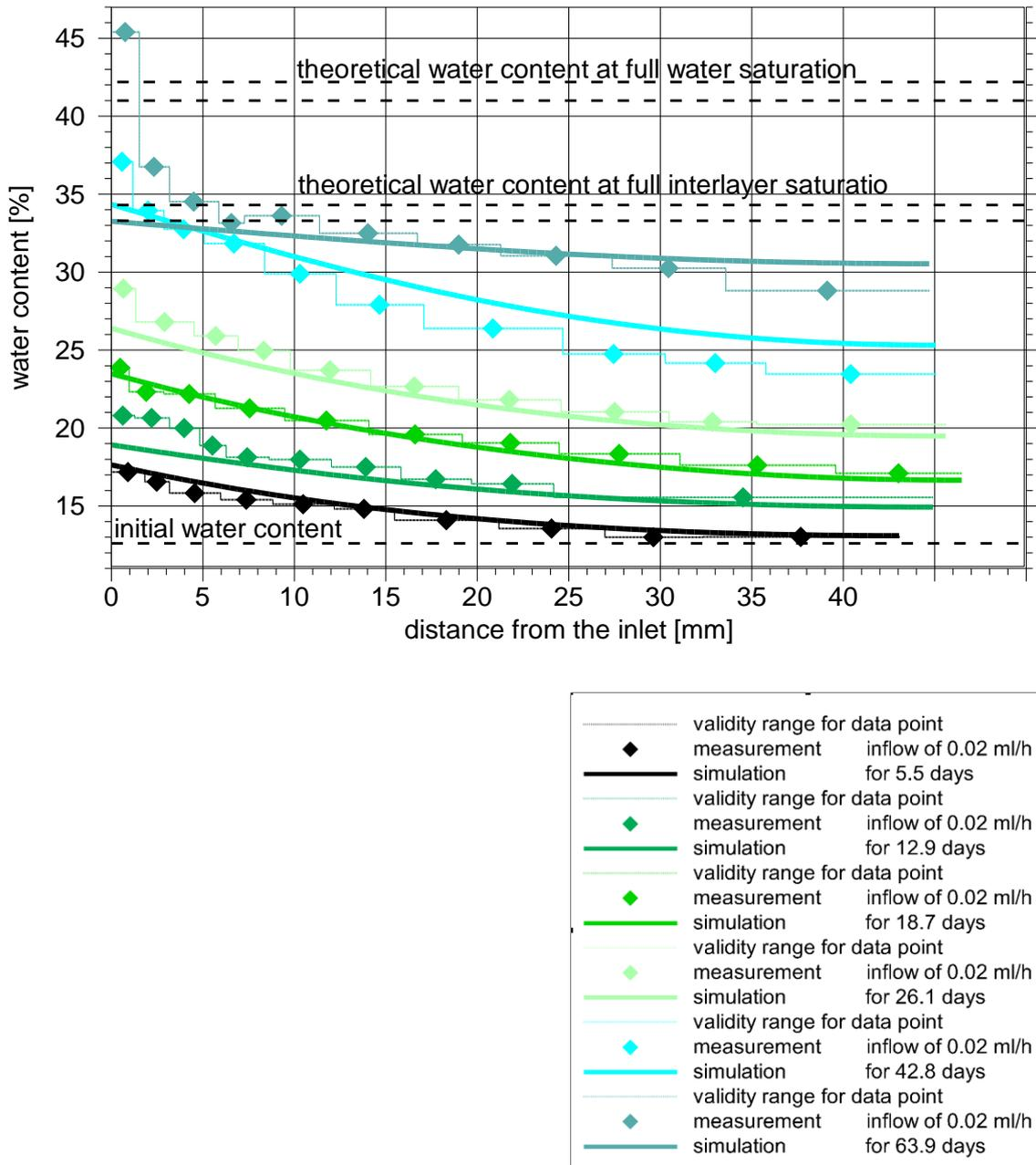
**Fig. 4.5** Measured and calculated water content distributions varying the running time
