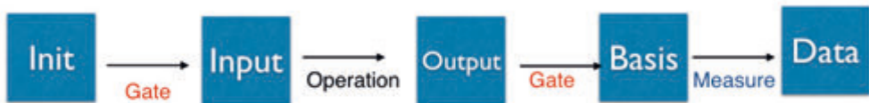
Fig. 4: SPAM errors in process tomography: The state that can be prepared and measured needs to be transferred into the basis that has to be prepared and measured, introducing additional errors obfuscating the channel.
