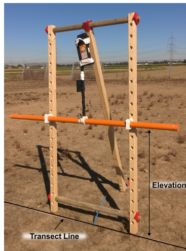
Figure 3.7: The measurement setup. A customized six coil CMD-MiniExplorer (GF Instruments, Czech Republic) is used with its Bluetooth handheld fixed to the crutch handle during measurements. The elevation was changed in steps of 0.2 m.
