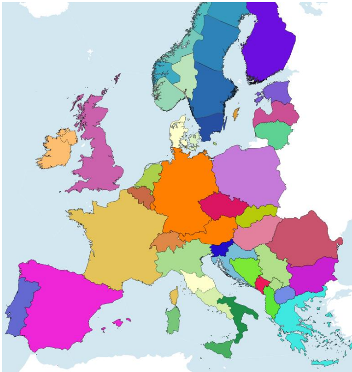
Figure 2-3 Configuration of the bidding zones in Europe. The only zone spanning more than one country consists of the Germany-Austria-Luxemburg zone. In each bidding zone a single price is applied uniformly after market clearing [39]. Own illustration.
