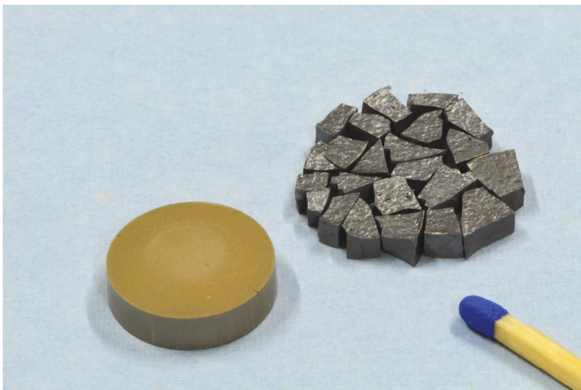
Figure 4-32 : Comparison of the FAST/SPS sintered pellets: (dark yellow and stable) with pressure less (PL) tool configuration under Ar/2.9%H 2 atmosphere and re-oxidation at 800°C and (black and fractured) with conventional pressure assisted (PA) tool under Ar/2.9%H 2 atmosphere [192].
