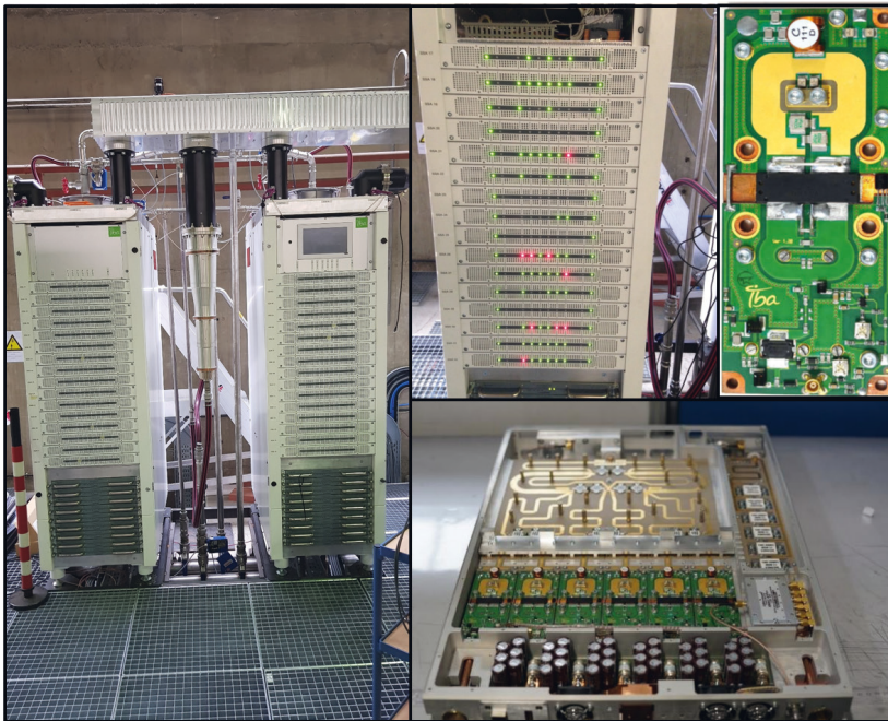
Figure V.23: 200 kW, 176.1 MHz Solid State Amplifier (SSA) developed for the MYRRHA project.
