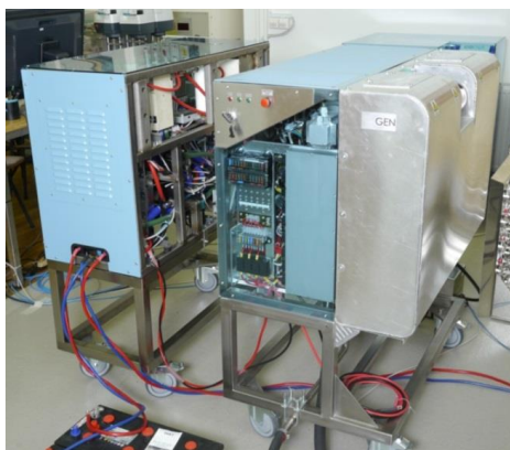
Fig. 30: FCGEN system with electric power of 3–5 kW; the fuel cell section is visible on the left, and the right-hand side shows the fuel processor
