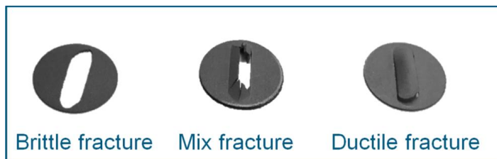
Fig. 56: Types of failure of sintered bodies
