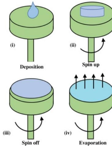
Figure 2.8: Stages of spin coating on substrate [107]
