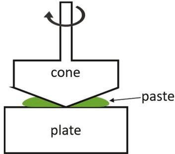
Figure 3.6: The scheme for a cone viscometer[135]
