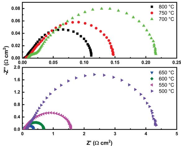
Figure 5.26: Impedance spectra measured from 800 °C to 500 °C
