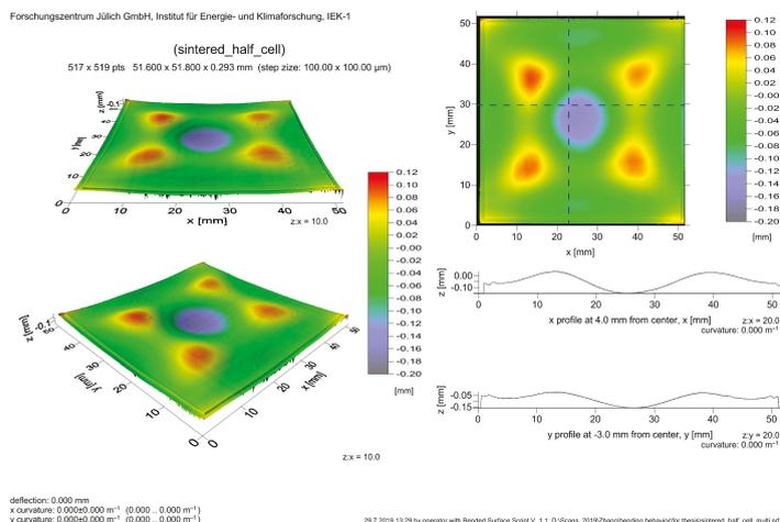
Figure 5.12: Topography measurement of the sintered half-cell
