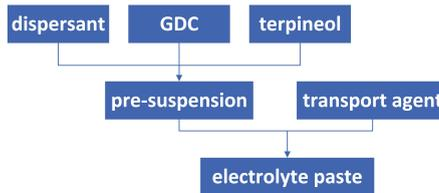
Figure 3.4: Process for the synthesis of screen printing paste for the electrolyte
