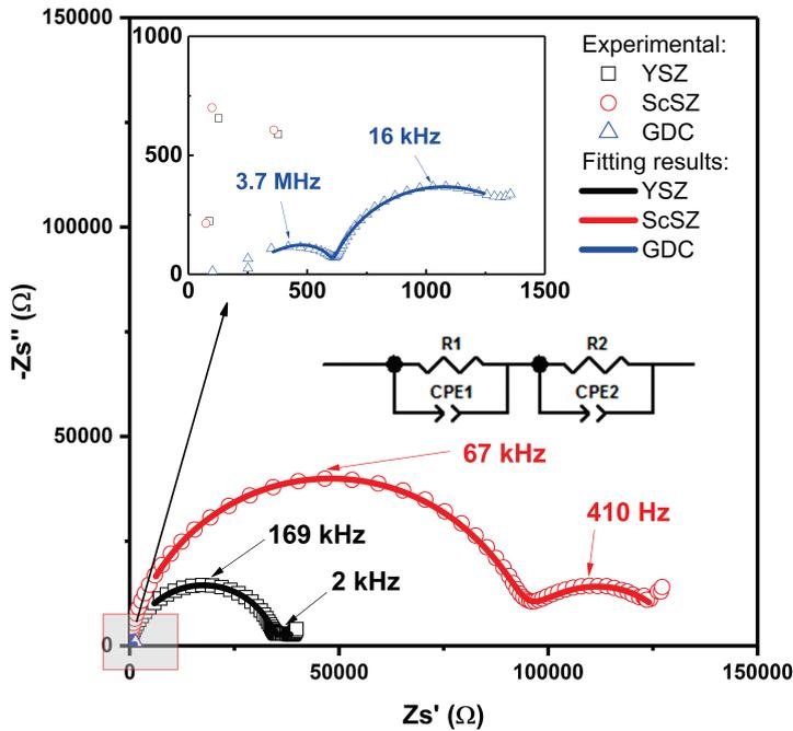
Figure 4.7: Typical impedance spectra of YSZ (black), ScSZ (red) and GDC (blue) at 300 °C. The experimental data are plotting in symbols and fitted data are plotting in lines
