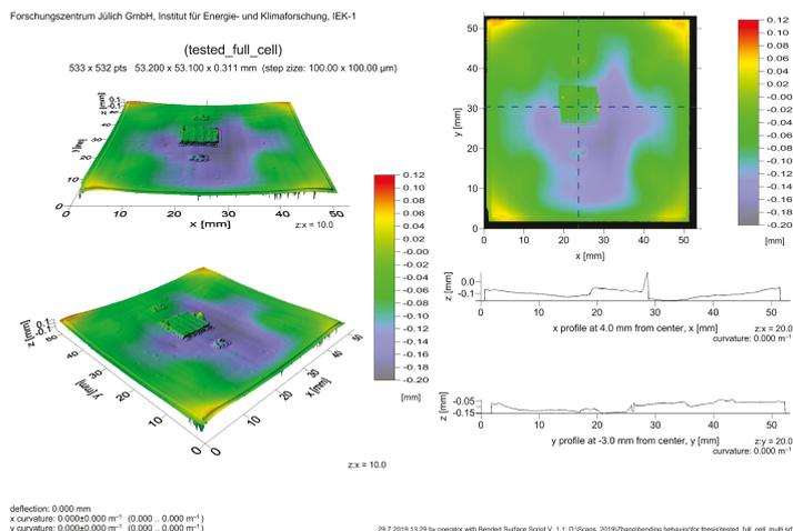
Figure 5.33: Surface topography of the tested full-cell
