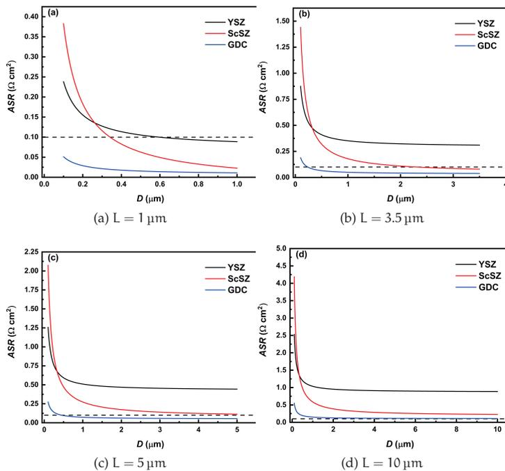
Figure 4.14: The dependence of  $\text{ASR}_{el}$  on the grain size for different fabricated electrolyte thickness  $L$  ( $T = 500^\circ\text{C}$ )
