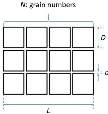
Figure 4.13: “Brick Layer” model of a poly-crystalline material, with grain boundary thickness of  $d$ , grain size of  $D$ , sample thickness of  $L$  and grain number of  $N$
