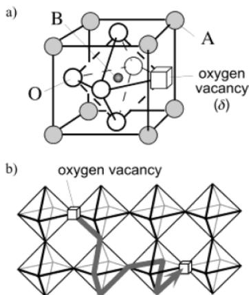
Figure 2.4: Atomic structure and oxygen transport in mixed conducting perovskites  $ABO_{3-\delta}$ . (a) Basic structure. (b) Bulk oxygen transport mechanism [32]
