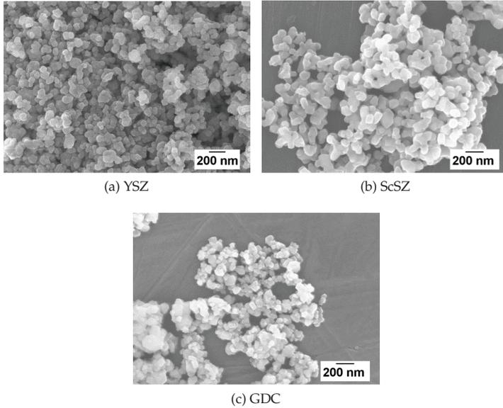
Figure 4.2: Raw powder morphology observed by SEM
