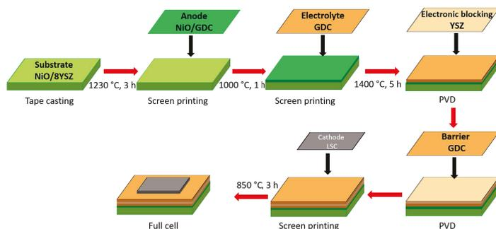
Figure 3.10: Manufacturing process of the full cell
