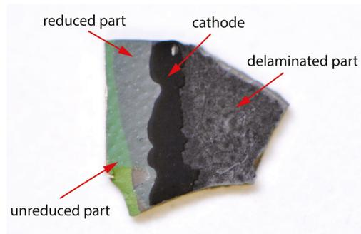
Figure 5.22: Optical photograph of a tested cell
