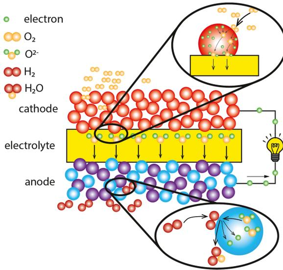
Figure 2.1: The working principle for SOFC
