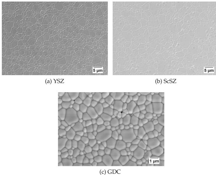
Figure 4.4: SEM cross-sectional microstructure for sintered pellets
