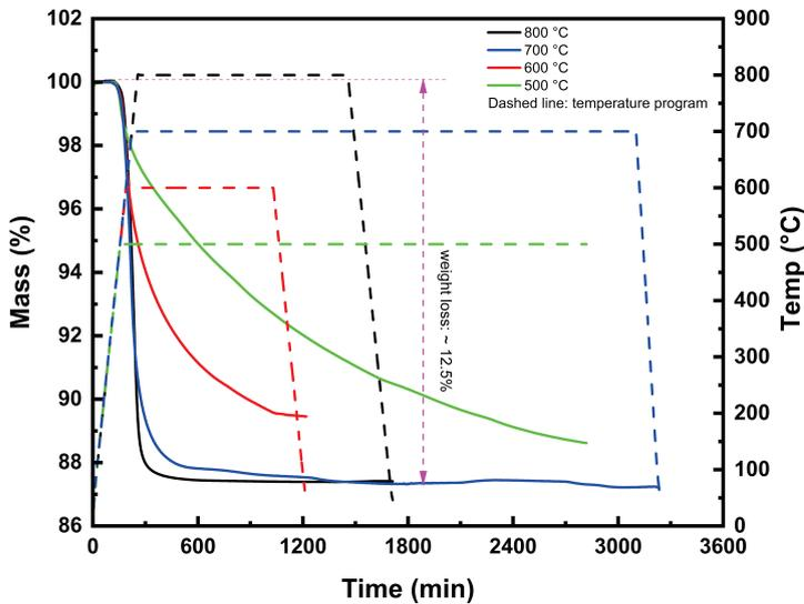
Figure 5.17: Thermogravimetric (TG) measurement for half cells measured under Ar/H<sub>2</sub> (2.9% H<sub>2</sub>) at different temperatures
