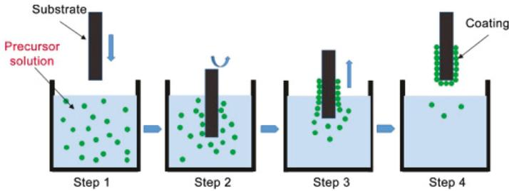
Figure 2.9: Graphical representation of dip-coating technique [110]
