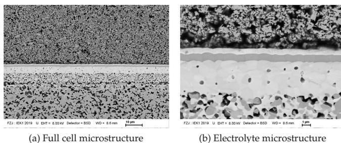
Figure 5.35: Cross-sectional SEM microstructure of the tested cell
