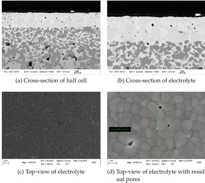
Figure 5.13: SEM images of the half-cell after sintering at 1400 °C for 5 h
