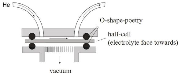
Figure 3.9: The leakage measurement scheme[138]
