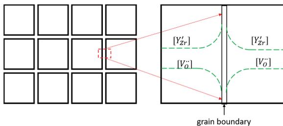
Figure 2.6: Left: Brick layer model of a polycrystalline material. Right: enlarged grain boundary with defect and oxygen vacancy concentration distributions (in green dash line)
