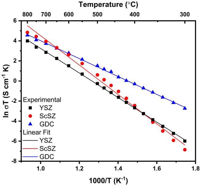
Figure 4.9: Comparison of experimental (denoted as symbol) and linear fit (as line) for YSZ (black), ScSZ (red) and GDC (blue)
