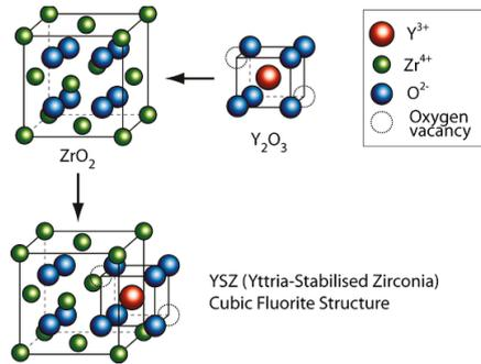
Figure 2.5: Oxygen vacancy formed due to the substitution of  $\text{ZrO}_2$  by  $\text{Y}_2\text{O}_3$  [47]
