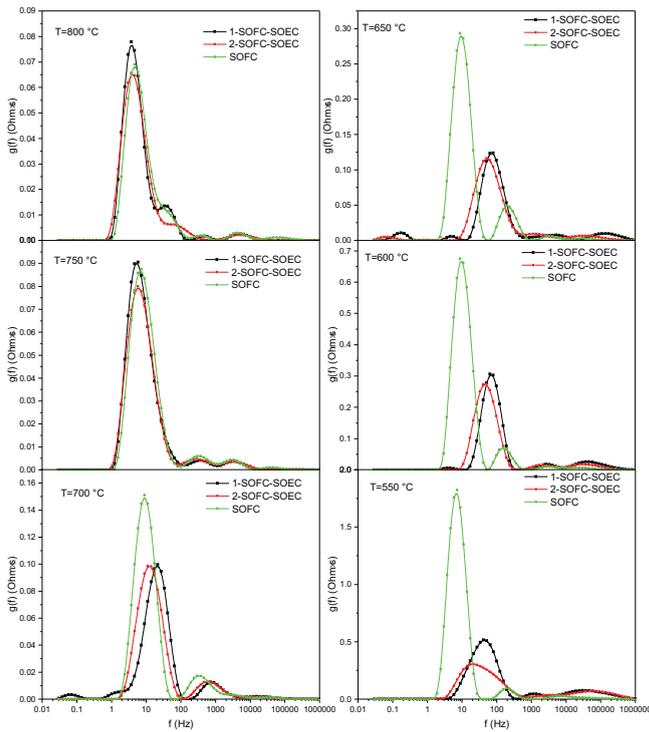
Figure 5.39: DRT comparison at different temperatures
