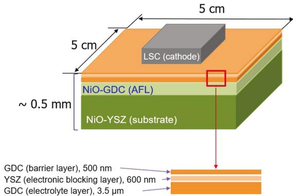
Figure 3.11: Schematic of full cell structure
