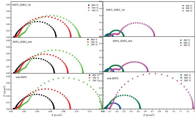
Figure 5.38: EIS comparison of SOFC and SOEC mode
