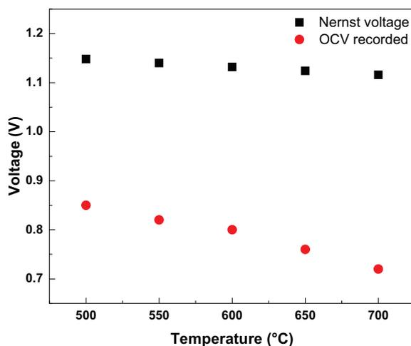
Figure 5.19: Cell voltage as a function of temperature
