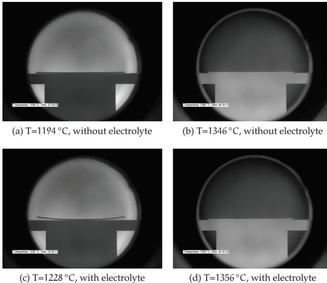
Figure 5.11: Comparison of warpage behavior during sintering
