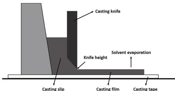
Figure 2.7: Scheme of tape casting process
