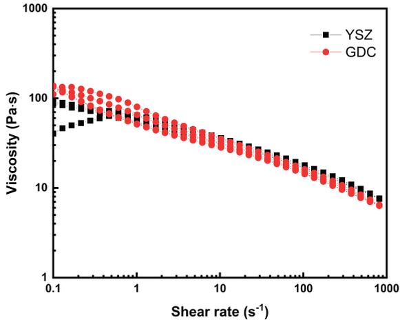
Figure 5.9: The comparison of viscosity between standard YSZ electrolyte paste and GDC electrolyte paste
