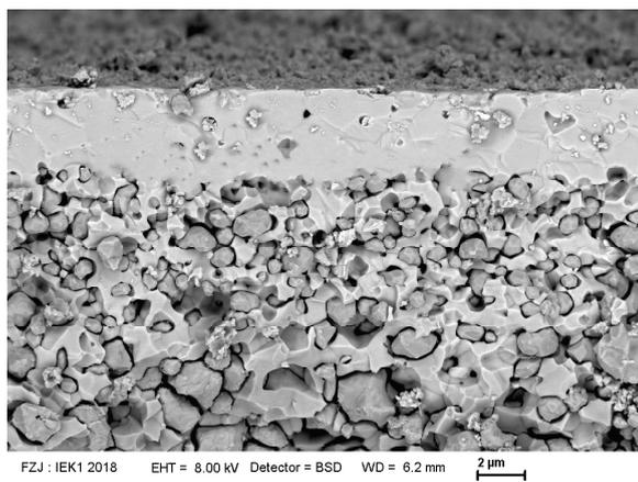
Figure 5.21: SEM fracture of full cell after single cell test
