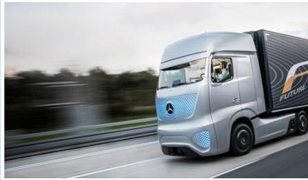
Mercedes-Benz has started testing its Future Truck 2025 with a self-driving system called Highway Pilot in 2014. After successfully testing the system on a closed-off road, German and U.S. (Nevada) authorities have permitted tests on public highways. The truck's intelligent driving system consists of radar sensors, a stereo camera and assistance systems such as adaptive cruise control, brake assist and lane keeping assist.
