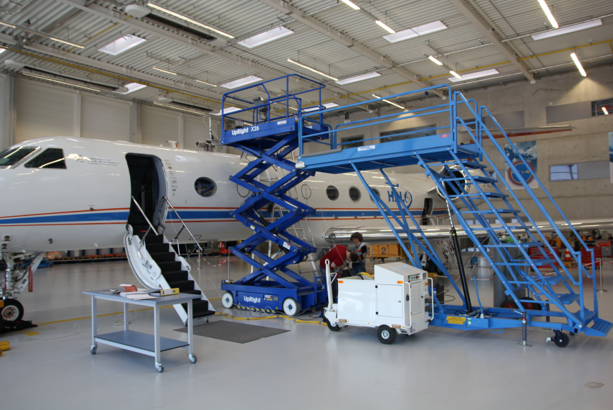
Figure 4.7: The OH and HO 2 inlets were on top of HALO and had to be accessed by a platform.
