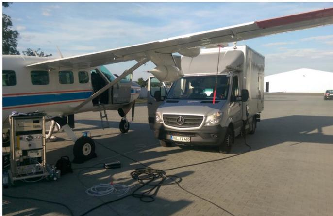
Fig. 2: Preparation for the outdoor air comparison at Schönefeld Airport (17.07.2018). Both air intake systems are positioned in close proximity to each other (Cessna: AIRPOD directly under the right wing; MobiLab: air intake at the head of the aerosol inlet). Appropriate positioning of the two systems ensured that contamination due to inherent emissions from the measuring platforms is avoided (wind-flow from the right).
