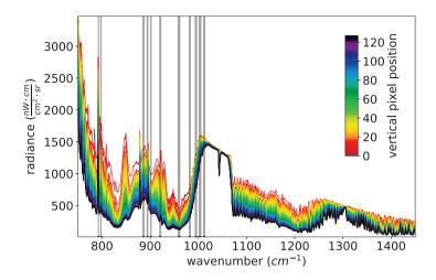
**Figure 3.2:** Infrared spectra measured by GLORIA on 25 January 2016 at 10:14 UTC. Shown are co-added spectra of the 128 superpixels. The spectral ranges used for the retrievals in this thesis (see Table 3.4) are highlighted in grey.
