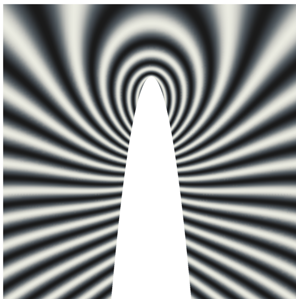
Fig. 8.4 Phase contour map simulated using an analytical line charge model. The phase contour spacing is \frac{2\pi}{12} radians. The white area denotes the needle itself. See text for details.
