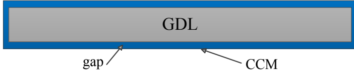
Figure 6.28: The sketch of fuel cells in which the CCM (MEA) is partially covered by the GDL (not to scale).
