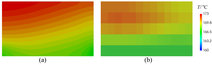
Figure 5.4: Temperature distribution, i = 0.6 \text{ A cm}^{-2} . (a) Numerical prediction by the DRA method; (b) Experimental measurements [99]. (Reproduced from [103])
