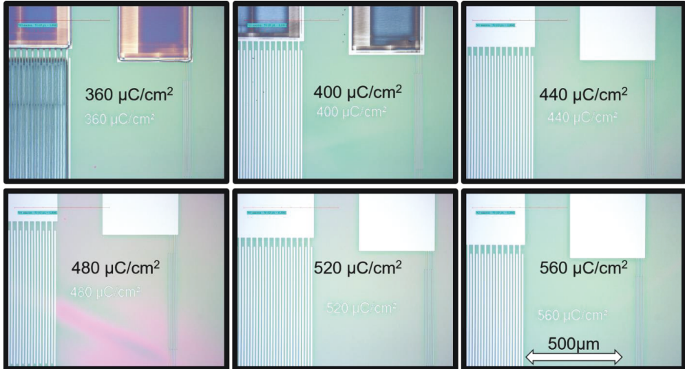
Figure 16: Optical microscope pictures of identical structures obtained for different doses of the 100 keV e-beam ranging from 360 \mu\text{C}/\text{cm}^2 to 560 \mu\text{C}/\text{cm}^2 .
