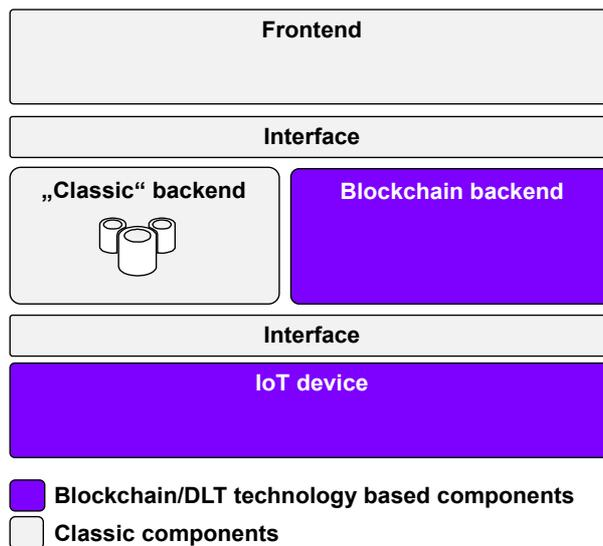
Figure 4: Technical architecture IoT tower
