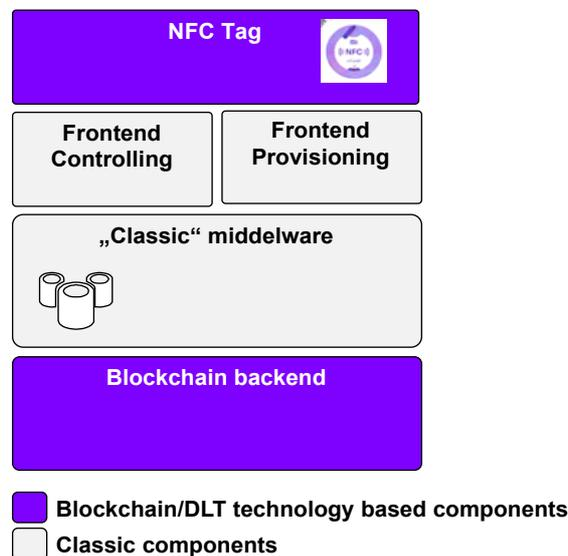
Figure 6: Technical architecture tagging final products
