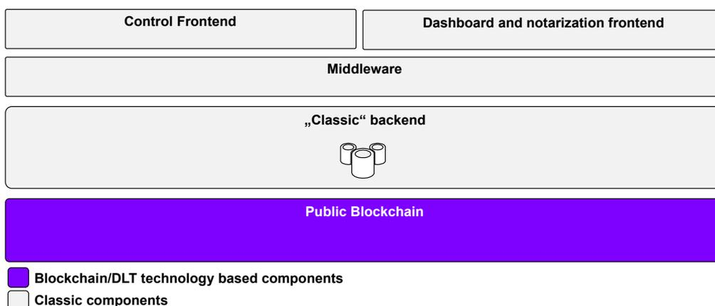
Figure 11: Technical architecture training and certification platform
