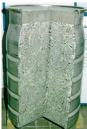
Figure 9 Drum containing encapsulated cladding waste (Fairhall and Palmer, 1997; Copyright © by WM Symposia. All Rights Reserved. Reprinted with permission).
