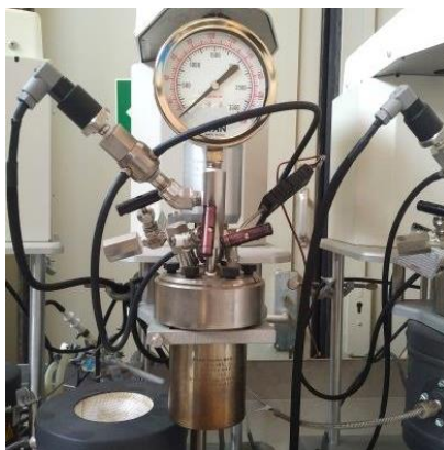
Figure 13 Parr autoclave used for alteration of cement and C-S-H phases under pressurized \text{CO}_2 conditions.
