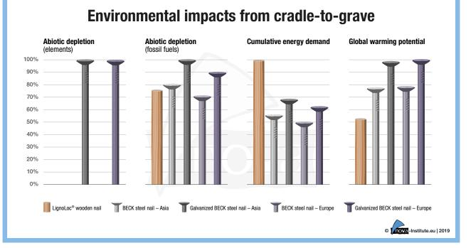
**Figure 4:** Environmental impacts of the LignoLoc<sup>®</sup> wooden nail in comparison to functionally similar steel nail variants from cradle-to-grave excluding use phase.
