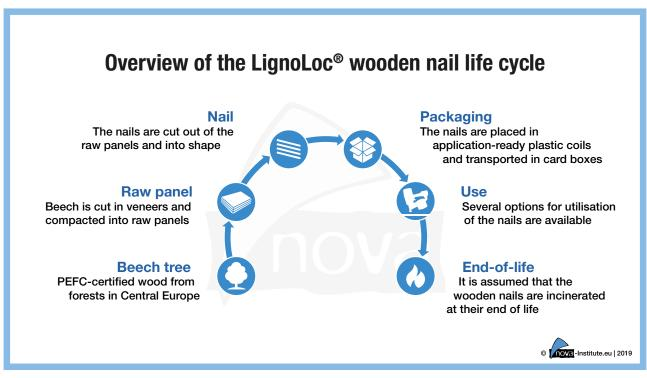
Figure 2: Overview of the LignoLoc® wooden nail life cycle
