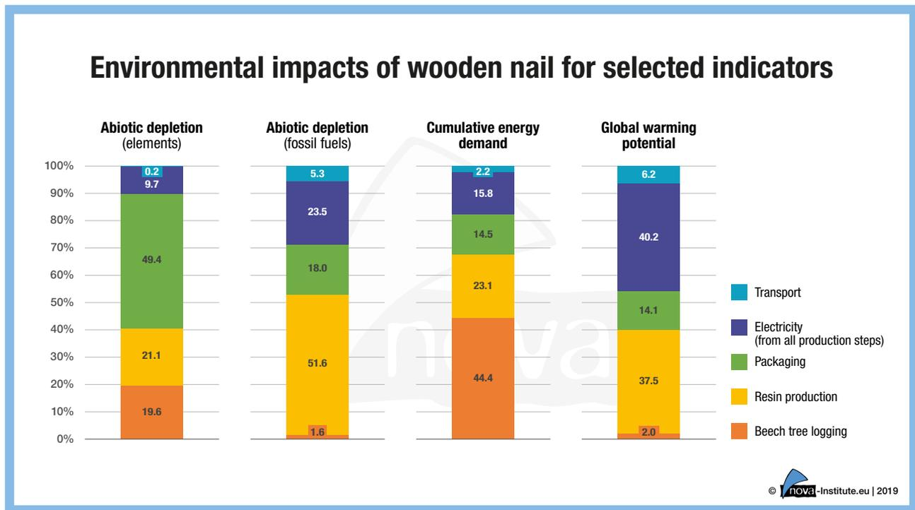
Figure 3: Hot spot analysis of the environmental impacts of the LignoLoc® wooden nail production (cradle-to-gate)
