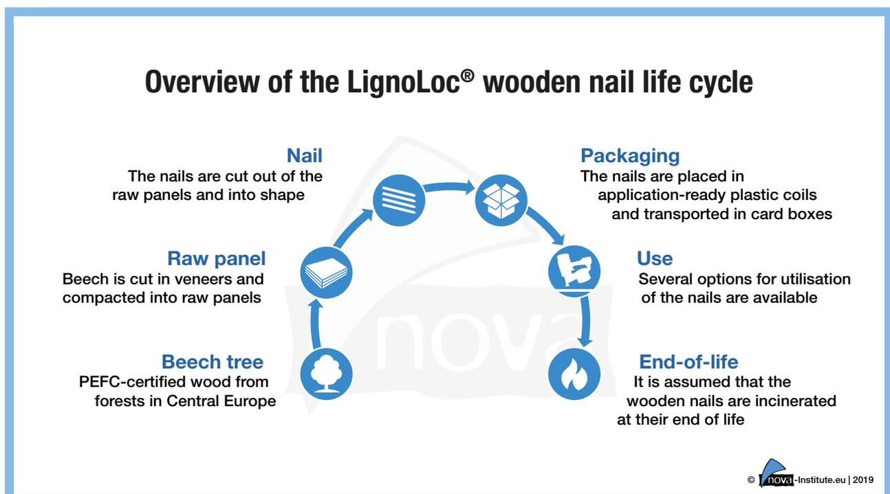
**Figure 2:** Overview of the LignoLoc® wooden nail life cycle
