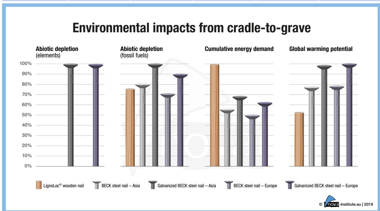
**Figure 4:** Environmental impacts of the LignoLoc® wooden nail in comparison to functionally similar steel nail variants from cradle-to-grave excluding use phase.
